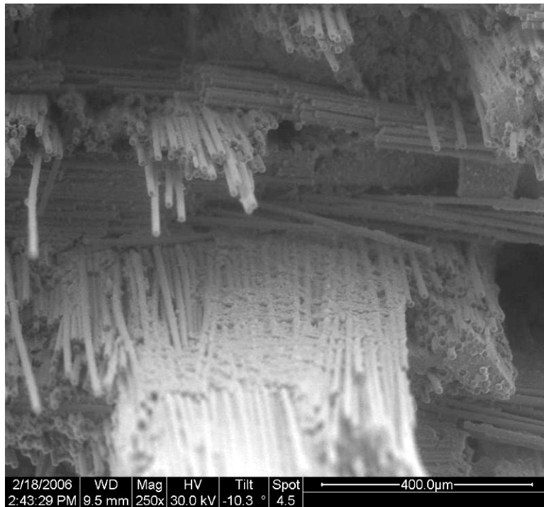
Figure 54. Specimen CH1 (notched, 125 MPa creep, 1200°C), 250x (hole 1.5 mm to left of image)
