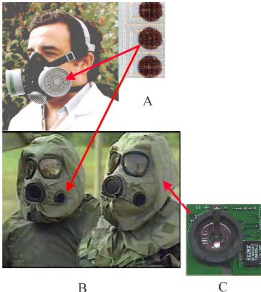
Figure 34: Cyrano Science’s prototype residual life indicators [106] (A) chemiresistors for respirator cartridges (B) the integration of chemiresistors or electronic noses to full body protection gear (C) electronic nose chip
