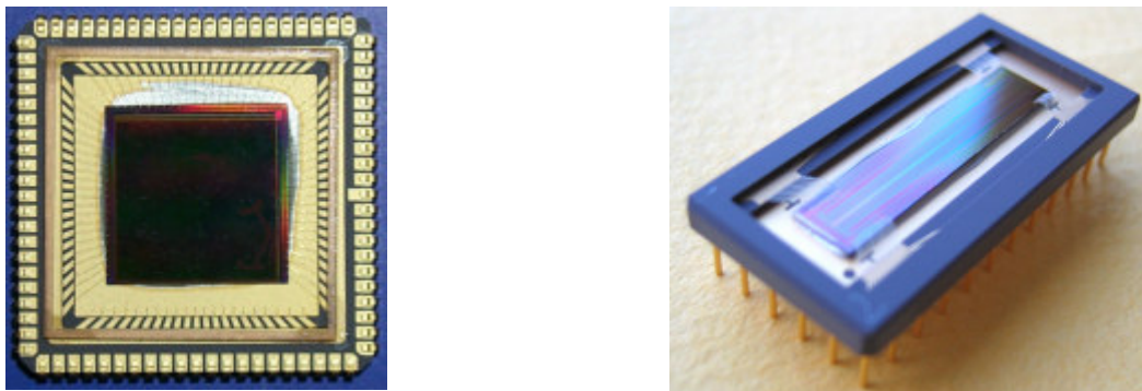
Figure 1 - Left: 1024x1024 pixels 2D array with 13 \mu\text{m} pixel pitch; right: 3078 pixels linear array with 6.5 \mu\text{m} pixel pitch: both devices have been manufactured using a 0.35 \mu\text{m} CMOS process optimized for imaging applications
