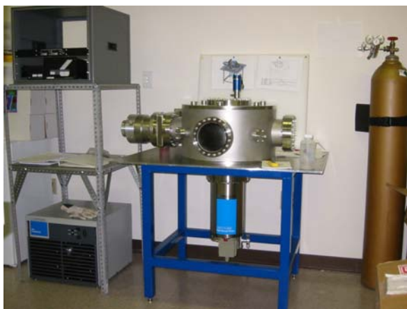
Figure 3.3-1A Cathodic arc deposition system.
