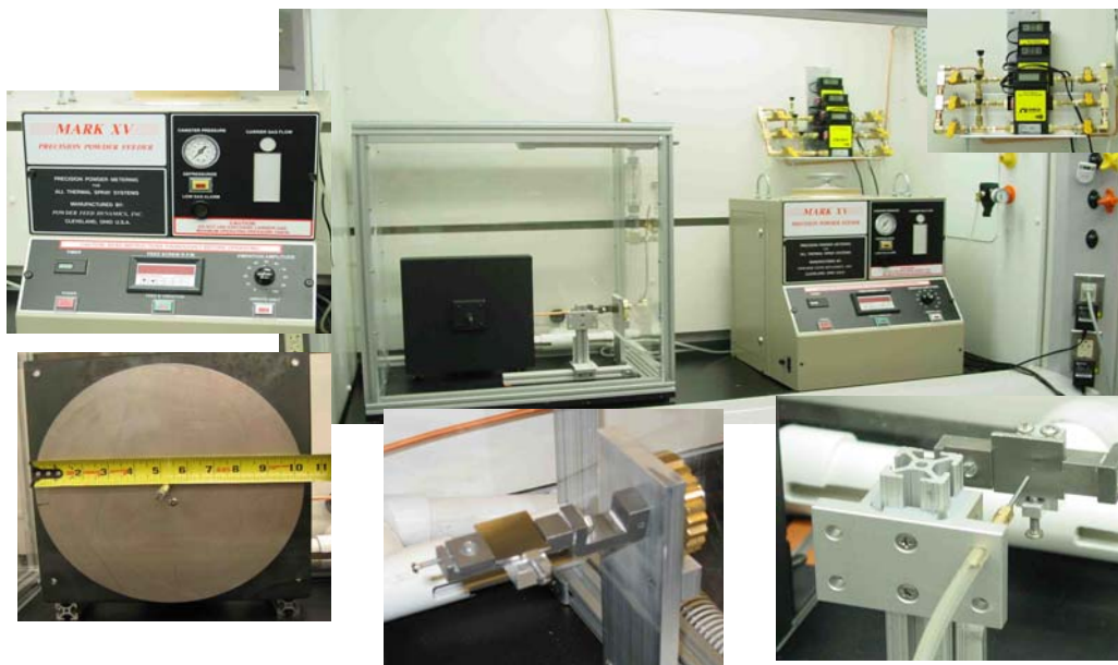
Figure 4.2-6. Gas Jet Erosion Tester – Final Version
