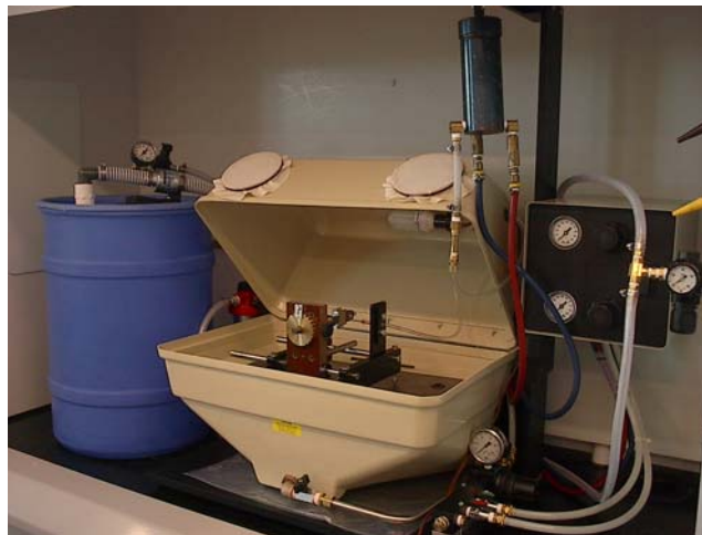
Figure 4.2-5. Gas Jet Erosion Tester – Initial Version
