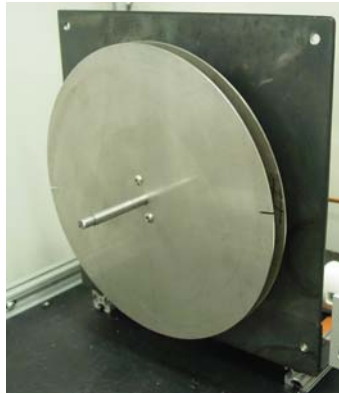
Figure 4.2-4. Picture of Double Disc Velocimeter – Final Version.
