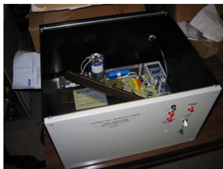
Figure 3.3-2. Cathodic arc pulse electronic power supply.
