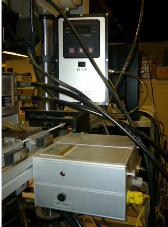
Figure 15: Water Pump and Steam Heating Unit
