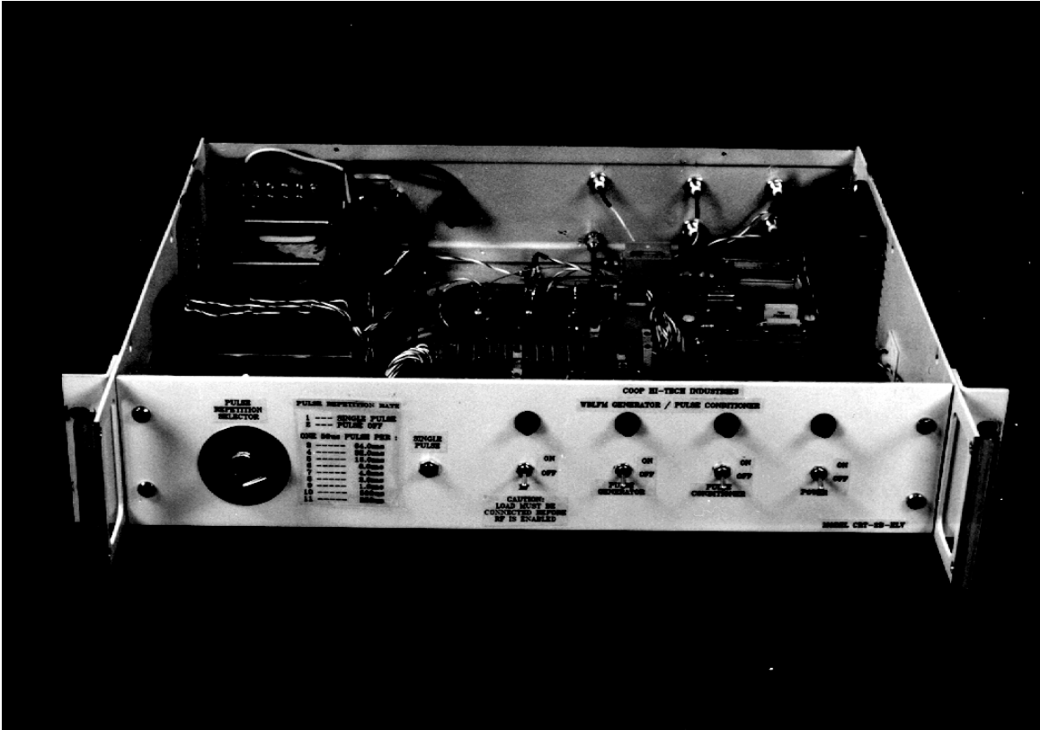
FIGURE 2.1.16 – PULSE CONDITIONER & LFM WAVEFORM GENERATOR
