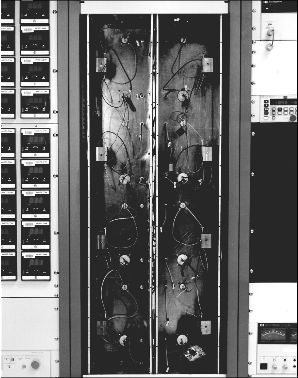
Figure 2.2.10 - LIFE TEST VERSION 2 DUT TEST CHAMBER
