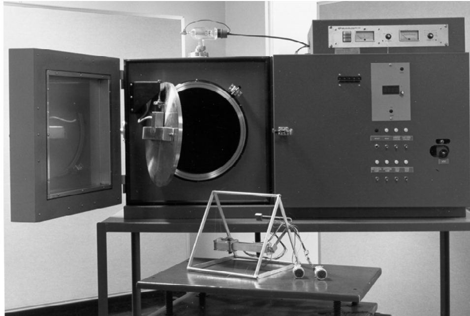
FIGURE 2.1.10 – SPACE CHAMBER WITH THERMAL TEST FIXTURE
