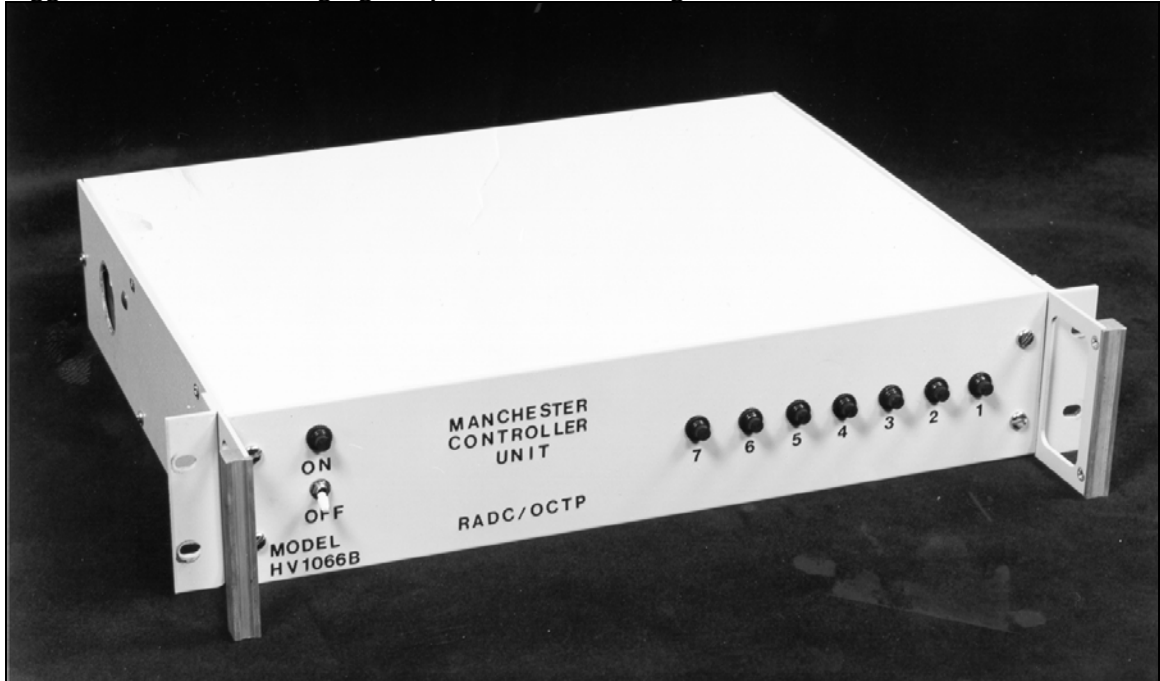
FIGURE 2.1.17 – C BAND MODULE CONTROLLER
