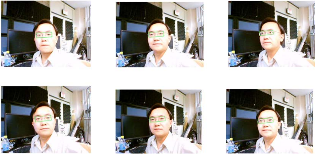
Figure 13: Sample frames of detected and tracked eyes from a video sequence captured by an active web-cam. From top-left to bottom-right: frame 1, 20, 40, 60, 80, and 100.
