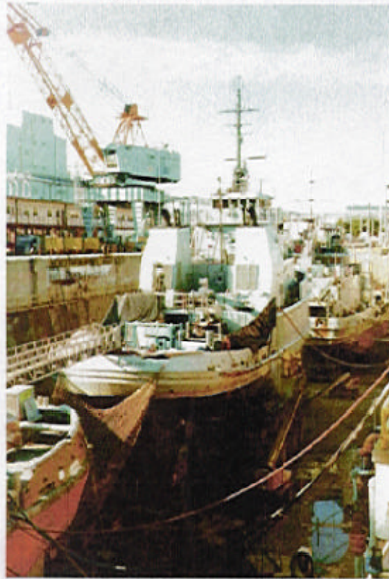
Figure 3: Workers on Hi-Lift using UHPWJ to remove paint from hull.
