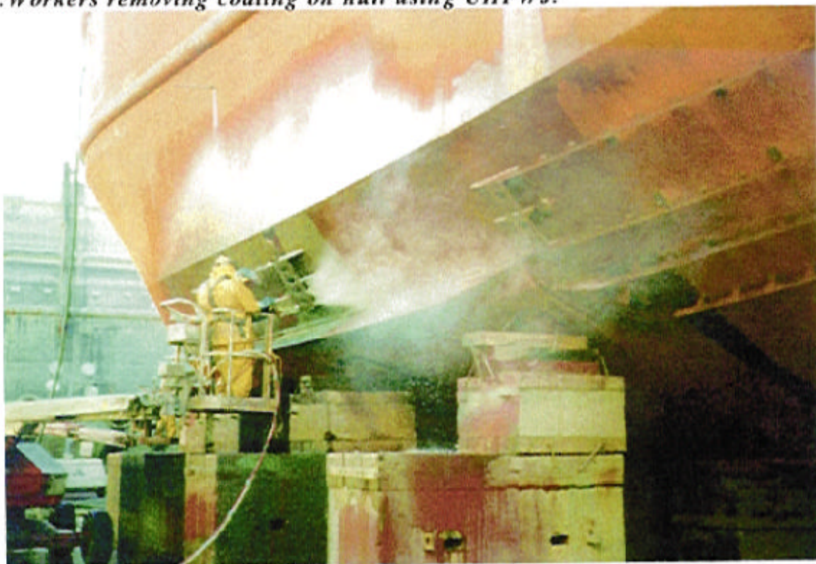
Figure 10: Workers removing coating on hull using UHPWJ.
