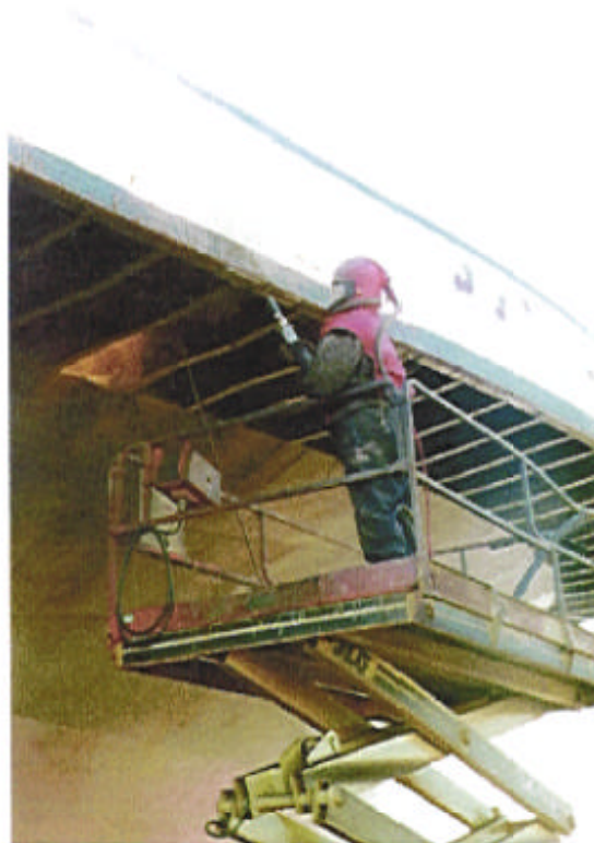
Figure 18: OAAB operator on Hi-Lift removing hull coating.
