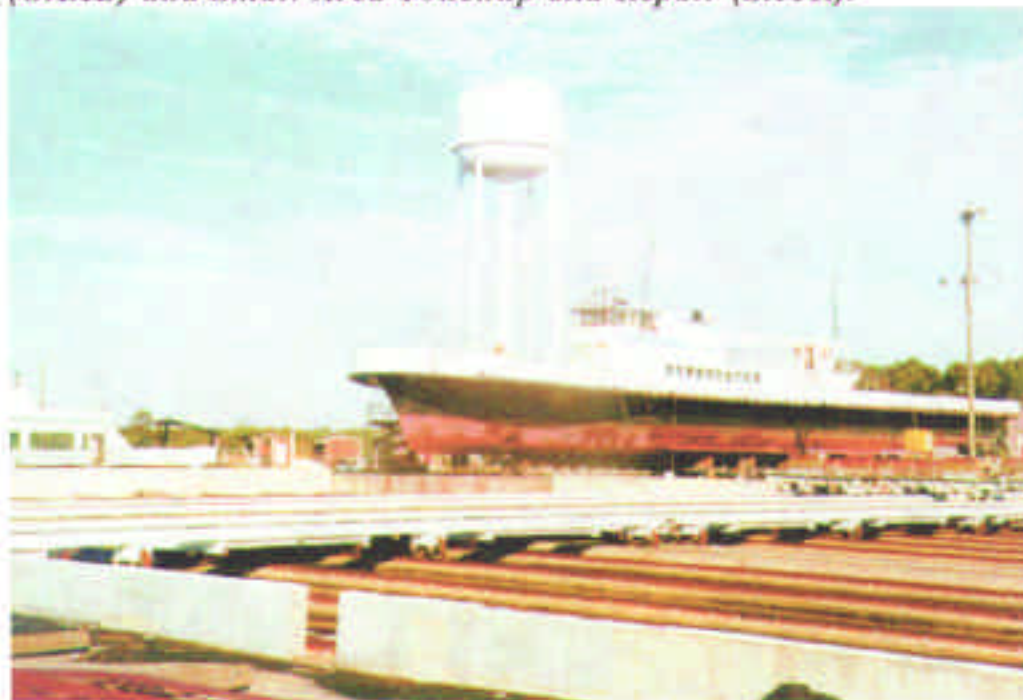
Figure 23: Ship having hull coating removed by Open air Abrasive Blasting (OAAB) and Small Area Touchup and Repair (SATR).
