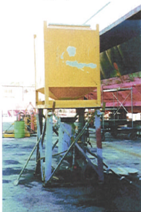
Figure 21:OAAB blasting pot filled with coal slag media.
