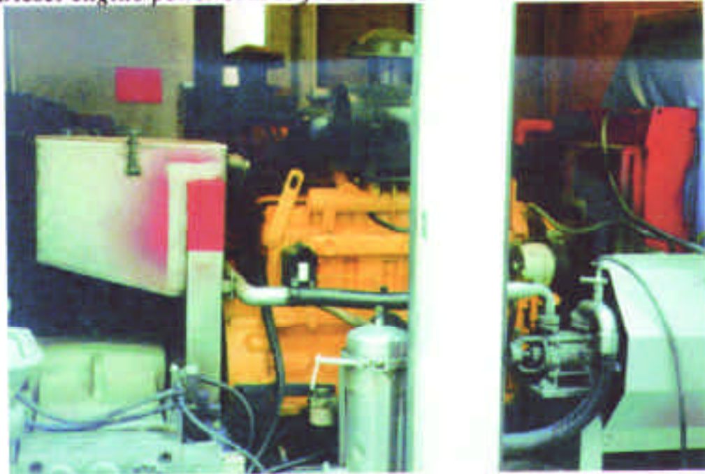
Figure 5: Diesel engine power source for UHPWJ.
