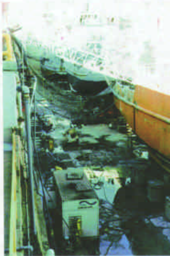
Figure 2: Ultra High Pressure Water Jetting (UHPWJ) equipment in dry dock.
