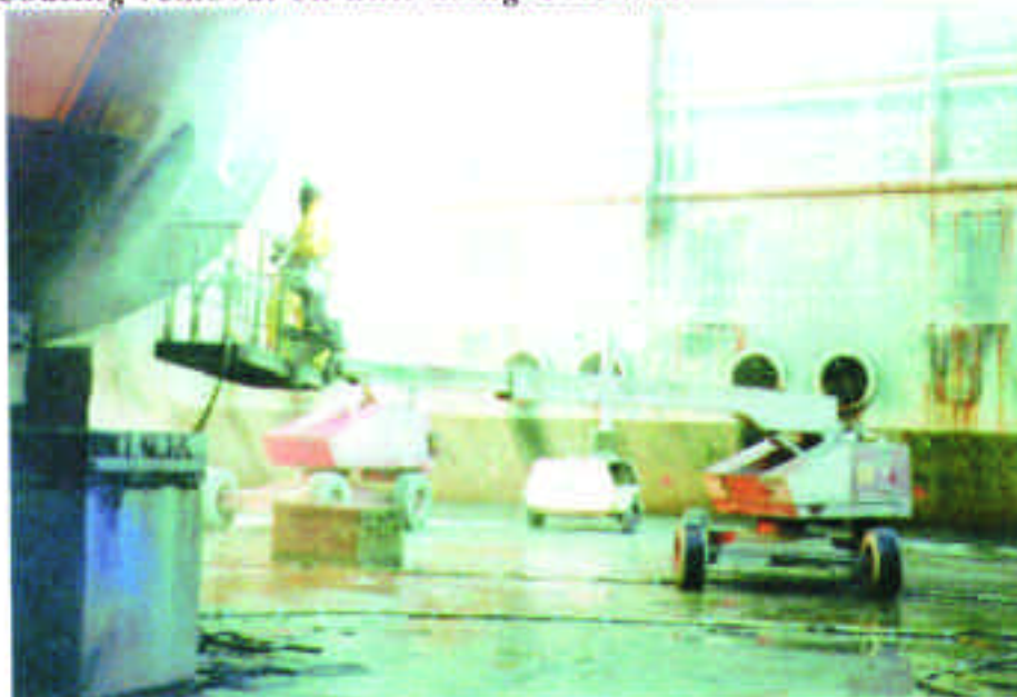
Figure 8: Operator and helper using UHPWJ
