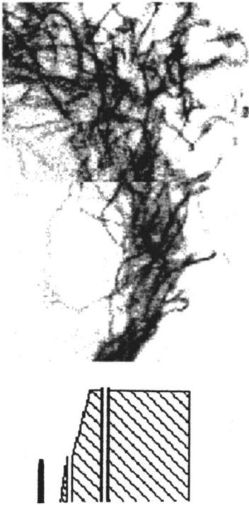
FIG. 5. Superposition of 25 images of CH layers showing the broad region in space over which the reaction layers move, due to turbulence. Imaged region is 46 mm high, 34 mm wide; left side of images is the centerline.
