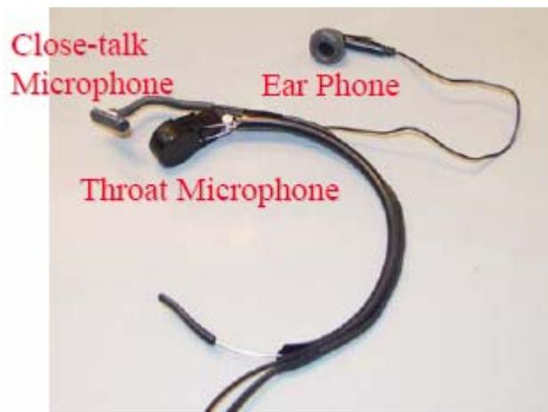
Figure 1.3. Throat and Air-Conductive Microphone (From [Zhang, 2004].).
