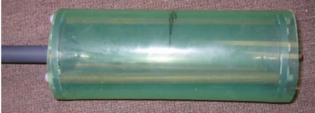
Figure 17. Conducting path with towed array tubing
