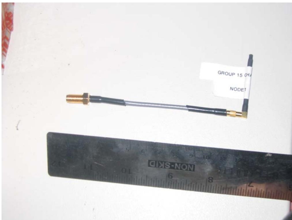
Figure 7. Mica-Z Antenna with Adapter.
