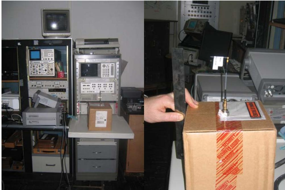
Figure 6. VSWR Measurement Setup.
