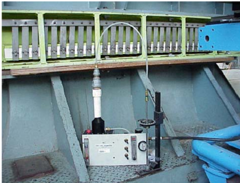
Figure 5. Six Jet Atomizer and Particle Seeding Probe [From Ref 7]
