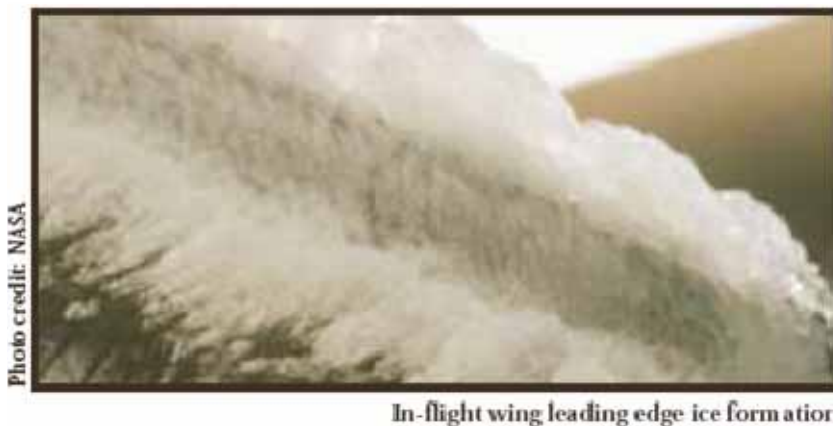
Figure 2. Leading edge mixed icing (from http://www.aopa.org/asf/publications/sa11.pdf 19 January 2006)
