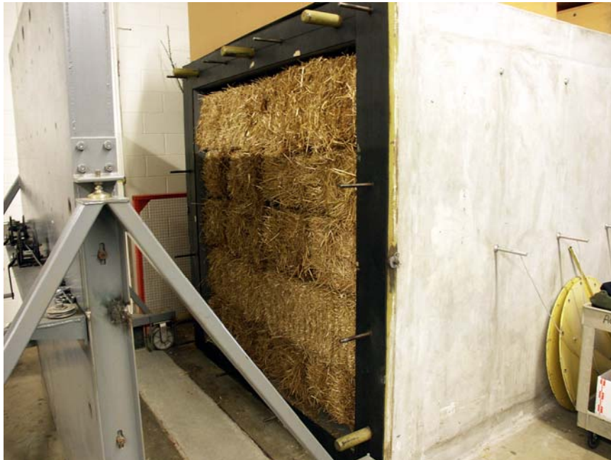
Figure 7.1 Ten bales of straw placed to terminate the empty chamber.
