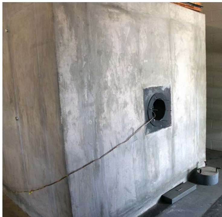
Figure 2.2 Loudspeaker installed in the center of the back of the chamber.
