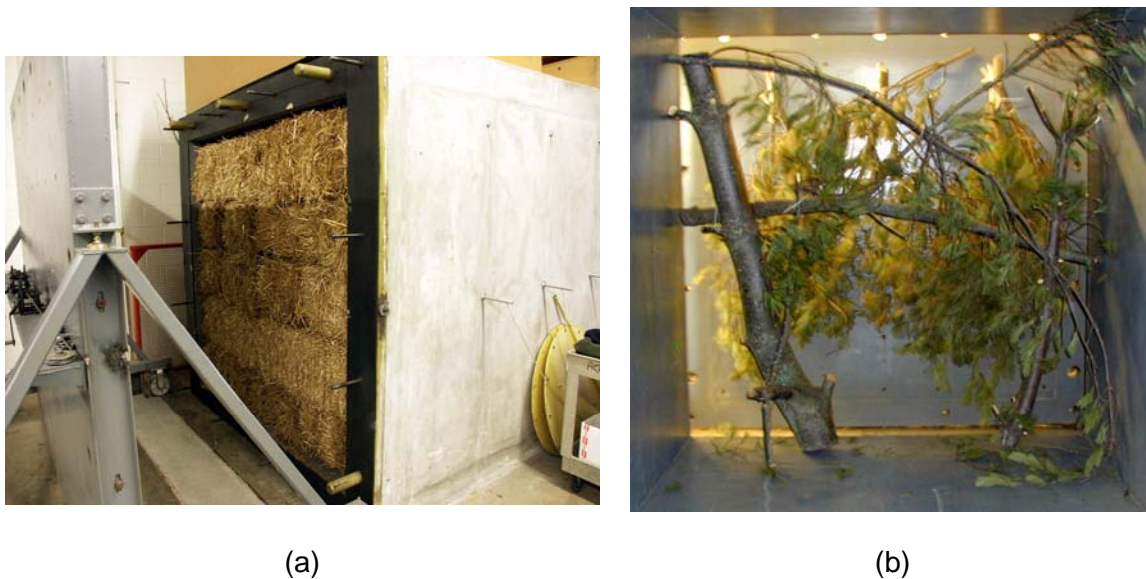
Figure 6.1 The chamber terminated with (a) 10-bale straw wall and (b) pine tree branches hung on the inside of the chamber door.
