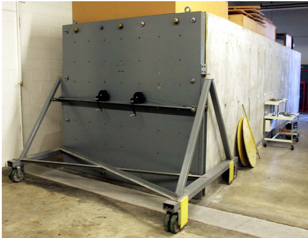
Figure 2.1 Reinforced concrete impedance chamber with steel door.
