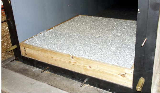
Figure 4.9 The lower half of the box filled with gravel.
