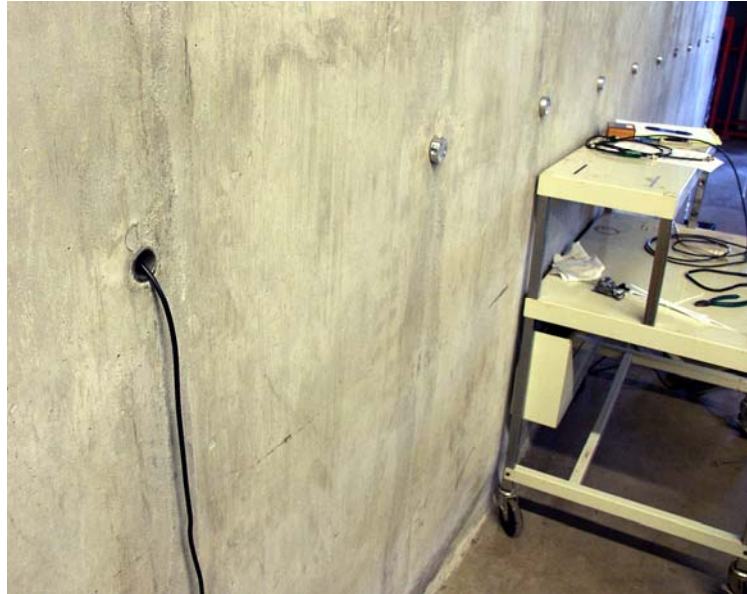
Figure 2.3 The microphone port on the left has a cable running out of it, whereas the other microphone ports are plugged.
