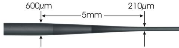
Figure 7 The image shows a side view of the taper section. The outer diameter of the fiber is reduced from 600\mu\text{m} to 210\mu\text{m} over a 5mm section. (Note: The image is stitched together from several images due to the limited field-of-view of the applied microscope).
