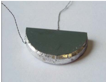
Fig.43. CCD photo of p-Ge scene (R=0.5 cm) with ohmic peripheral contact R 2 and p + central contact R 1 . In the accumulation mode, all carriers generated inside “broad” base concentrates in the vicinity of small central contact by giving rise to high positive apparent temperature. In the exclusion mode, free carriers are easy to recombine at broad ohmic contact by making the entire base “cold”.
