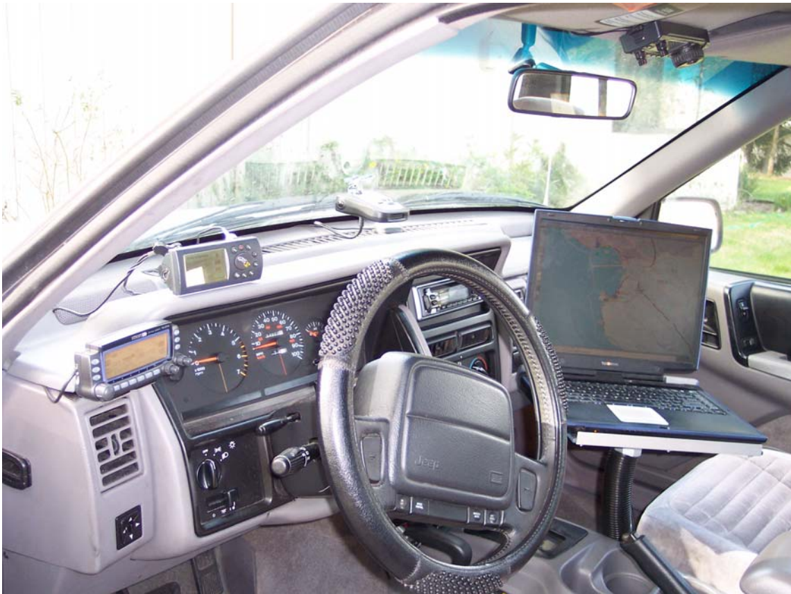
Figure 24. AE6QE-7 APRS Station with Computer Installed
