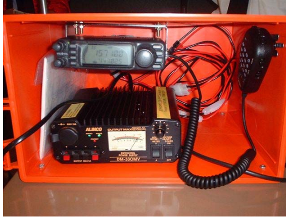
Figure 28. Emergency Communications Portable Solution (from: The Box: Portable Emergency Communications Station Ideas)
