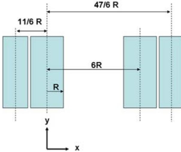
Figure 3. Augmented Railgun Geometry where  $R = 3/16"$
