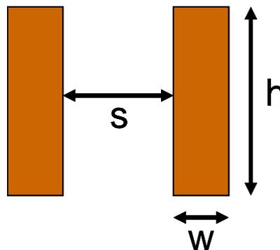
Figure 30. Kerrisk's Method Rail Parameters [After Ref. 2]
