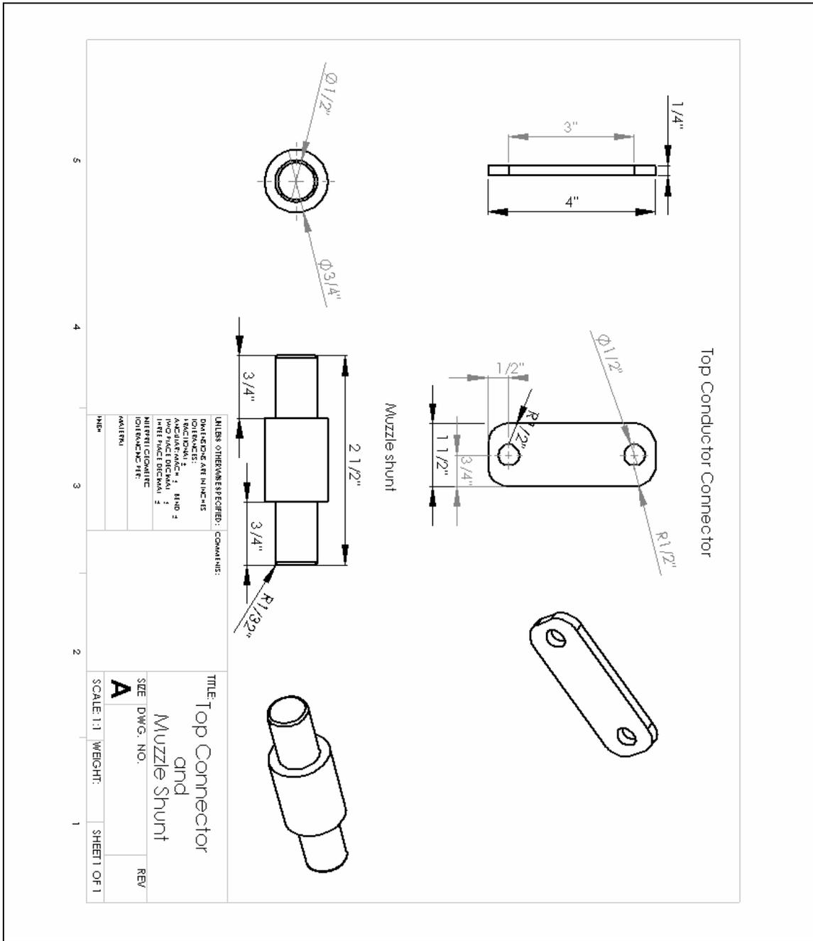
Figure 21. External Conductor Connectors and Muzzle Shunt
