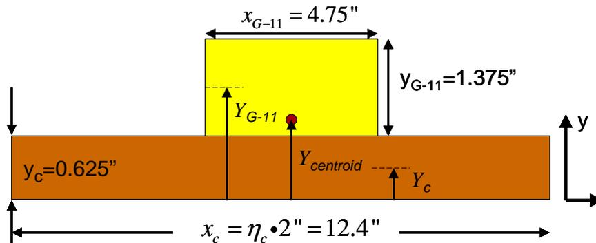
Figure 32. Transformed Homogenous Beam Geometry (Not to Scale)
