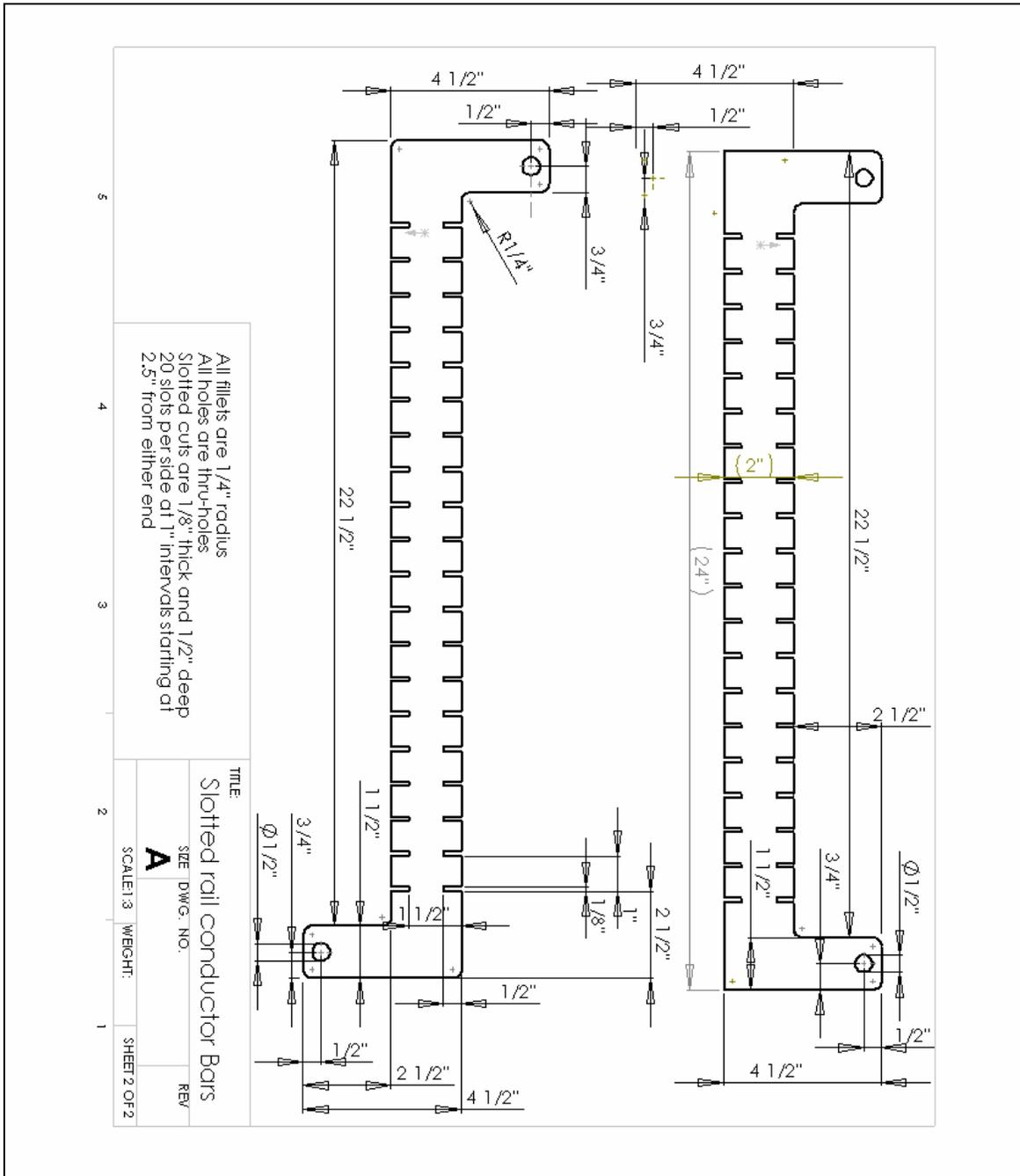
Figure 17. Slotted Primary Conductor Rails
