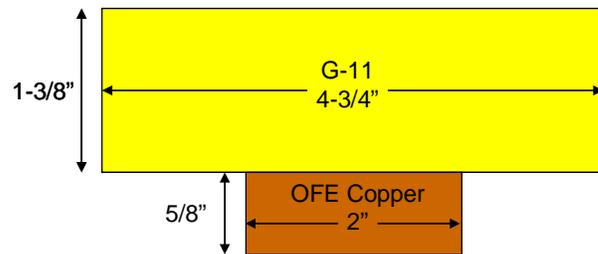
Figure 31. Simplified Beam Geometry (Not to scale)
