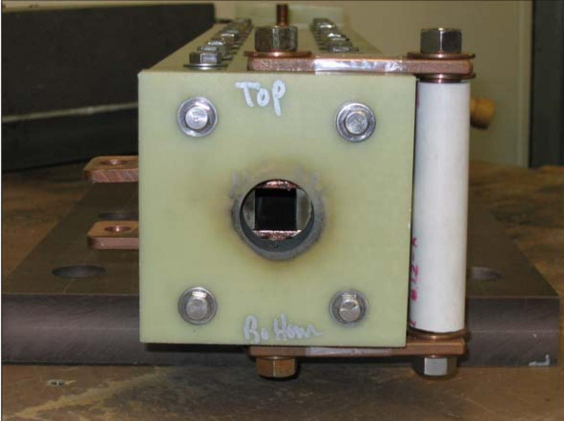
Figure 59. Muzzle Block Indicating Muzzle Flash Arcing
