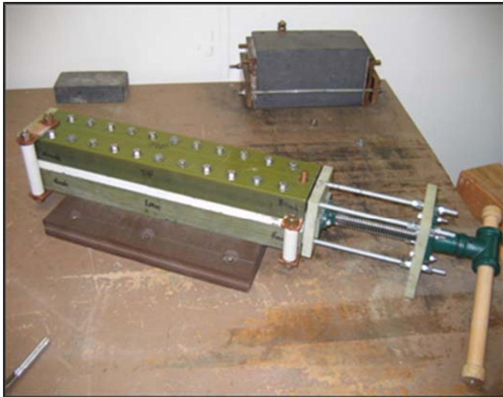
Figure 24. Full Assembled Railgun with Loader
