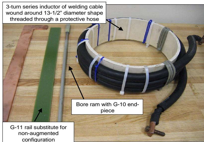
Figure 7. 3.0- $\mu$ H Series Inductor and Components
