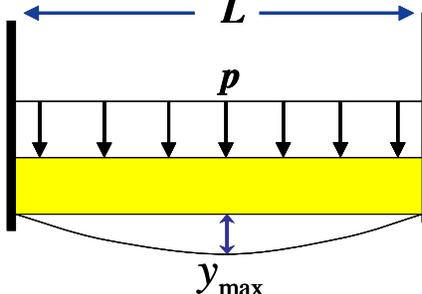
Figure 11. Fixed End Distributed Load Beam Model [After Ref. 9]
