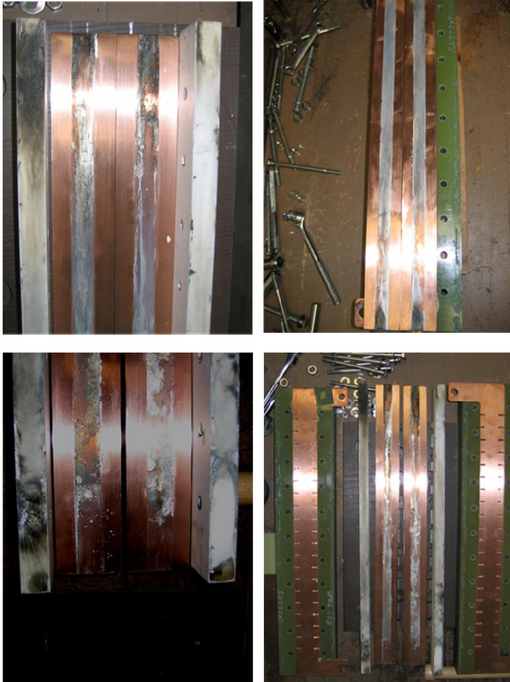
Figure 57. Typical Post-Shot Rail and Insulator Wear
