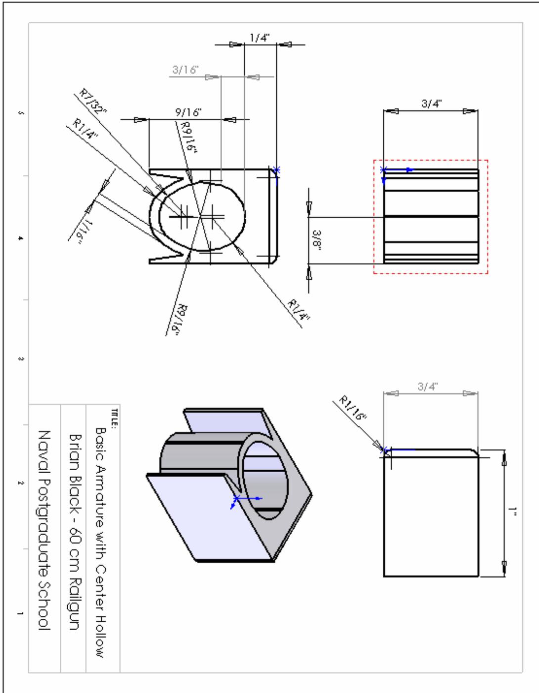
Figure 28. Altered U-shape Armature with Center Hollow
