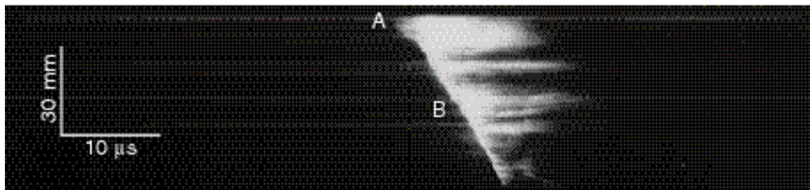
Figure 1.30. Streak record of a type II deflagration-to-detonation transition in ultrafine PETN. A - Point at which initiation takes place; B - Detonation wave travelling at 5.6 \pm 0.3 \text{ mm } \mu\text{s}^{-1} .
