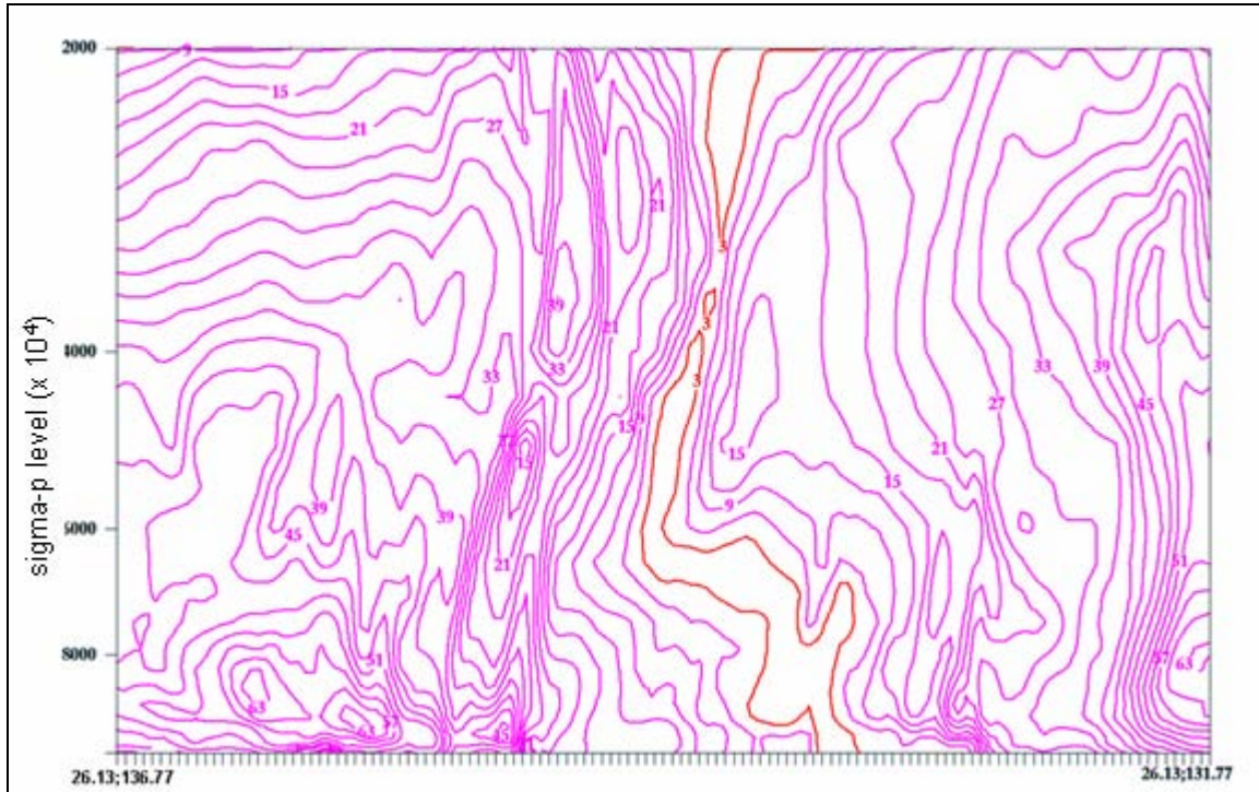
Figure 4.10 West-to-east cross section of normal wind component (kt) for the 72-h ARW inner nest forecast from the second Typhoon Nabi integration. Shearing of the storm caused the upper-level circulation center to be displaced from the low-level circulation center, which resulted in a significant error of the ARW vortex tracker. The horizontal interval is approximately 2.2 n mi.
