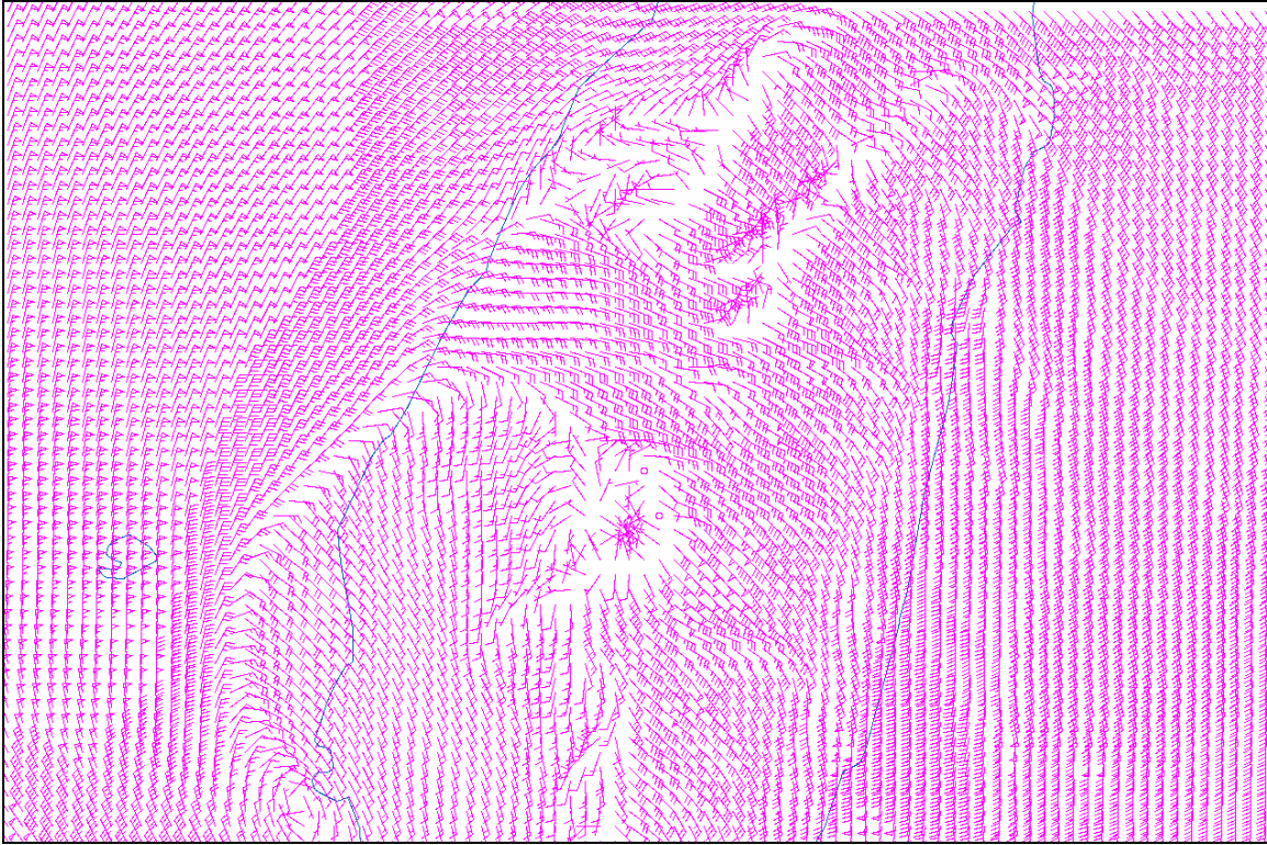
Figure 4.11 10 m wind barbs (kt) over Taiwan from the 66-h ARW inner nest forecast of the second Typhoon Talim integration. The winds are displayed at every grid point. The vortex center of Talim is in the lower left of the image, just off the west coast of Taiwan. Several mesoscale circulations were created by the terrain in the ARW, and may have helped create 500-mb height perturbations wthat caused an error in the vortex tracker algorithm.
