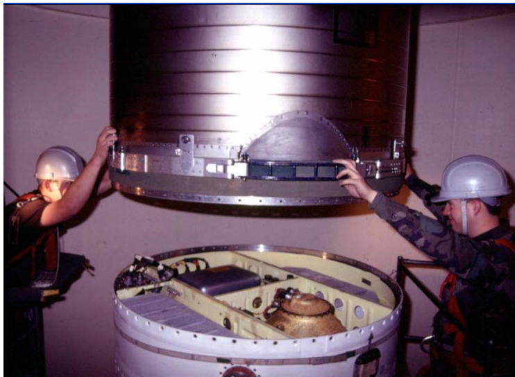
Figure 18: Minuteman III Reentry System Install (LGM 30 Minuteman III)
