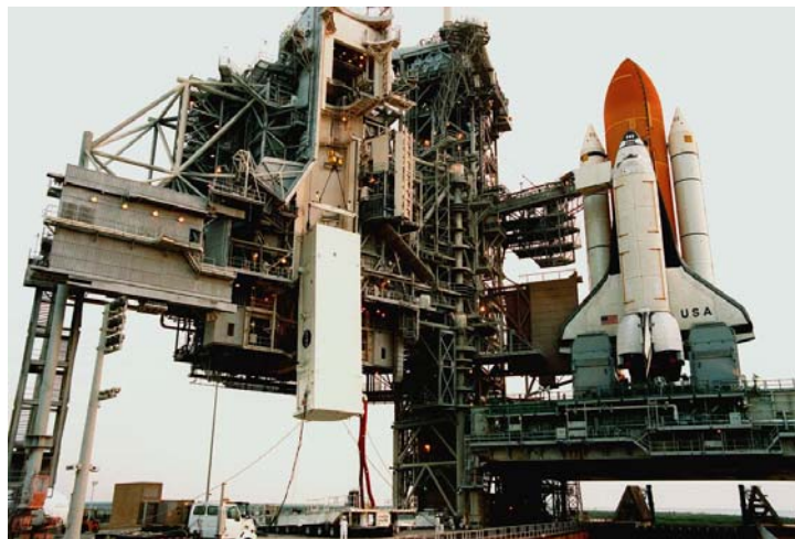
Figure 13: Payload installation operations at the launch pad (Cates, 2003:126)
