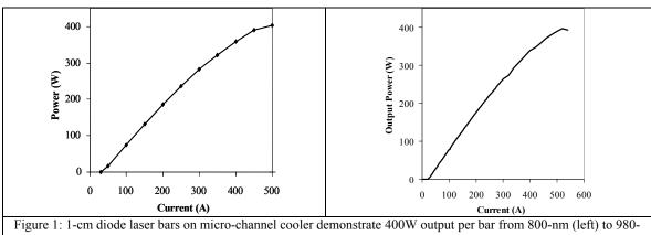
nm (right). Cavity length is 3-mm, fill factor is 80% and water is at 6-°C with 0.5lpm flow rate
