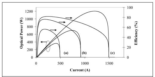
Figure 5: Extrapolated maximum power from a single 1-cm diode laser bar on micro-channel cooler (a) model fitted to measured 364-W, 58% efficient 800-nm material [4] (b) expected performance if thermal resistance is reduced to 0.2-°C/W and efficiency increased to 76% (c) expected performance for 0.14-°C/W and 80% efficiency [2].
