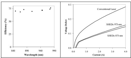
Figure 8: (Left) High efficiency > 70% is measured for 200-μm stripe, 1-mm cavity single emitters on c-mount at 25-°C from 850-nm to 980-nm. (Right) the high efficiency relies on low voltage defect [3], which is sustained from 850-nm to 975-nm.
