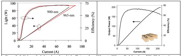
Figure 9: (left) 1-cm diode laser bars show high efficiency from 900-nm to 980-nm. Both bars have 25% fill factor, 1-mm cavity and are mounted on micro-channel cooler with 5°C water at 0.5-lpm. Peak efficiency was confirmed by NIST. (right) 980-nm material achieves peak efficiency of 73% [2].
