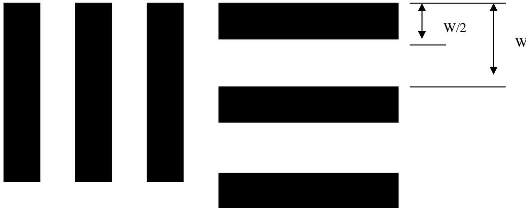
Figure 9. Example of lines in standard target. Note "W" is one cycle, i.e. the distance from the edge of one black line to same edge of the next back line.
