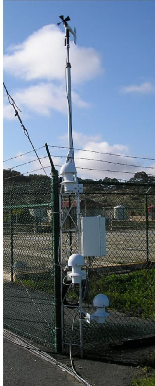
Figure 2. Meteorological tower deployed at Del Monte Beach, near optical target.
