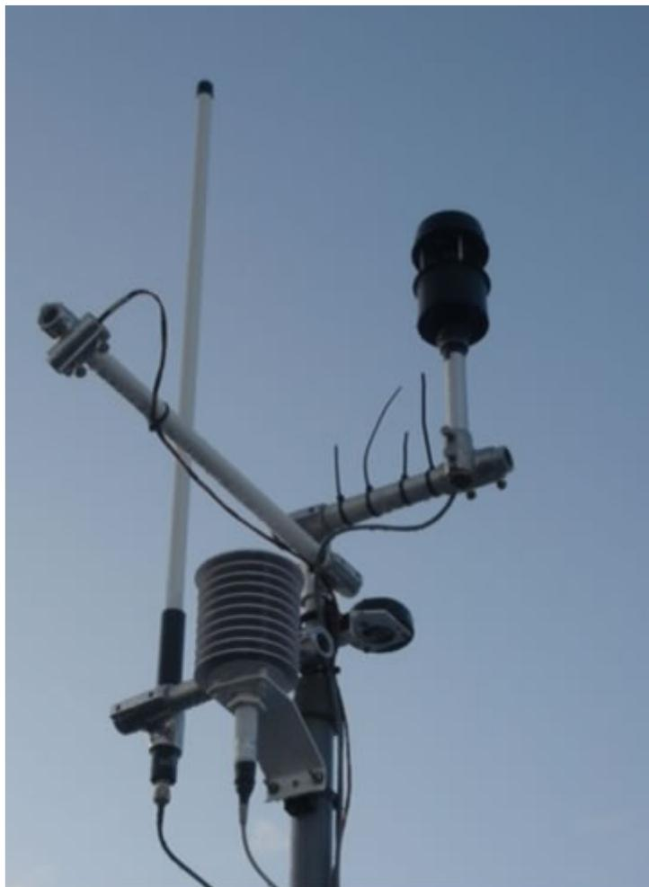
Figure 1. Photograph of meteorological sensors and communication antenna mounted on *Cypress Sea* during TNT 05-3.
