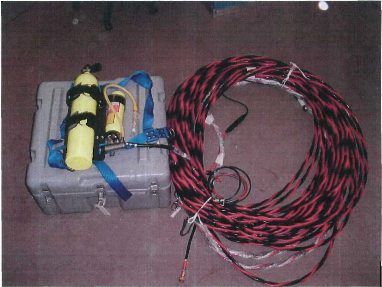
Photo 1. Dive Lab XLDS RDC-3 console with one 300-foot umbilical. The diver-worn harness includes two cylinders. The larger cylinder is the emergency gas system (EGS). The smaller cylinder is the intermediate compensating system (ICS). The high-pressure whip assembly used to supply HP breathing gas from scuba cylinders is not shown.
