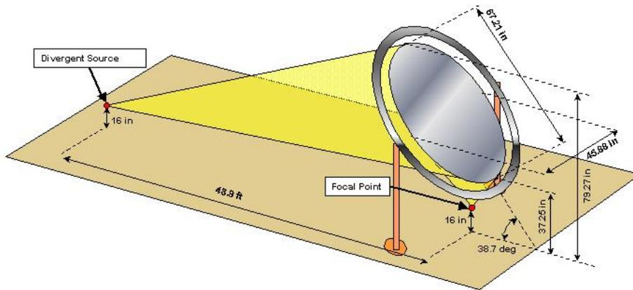
Figure EX1 Test Setup.
