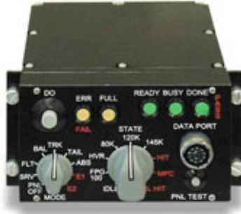
Figure 8.3 VMEP Vibration Monitoring Unit – Data Acquisition Device
