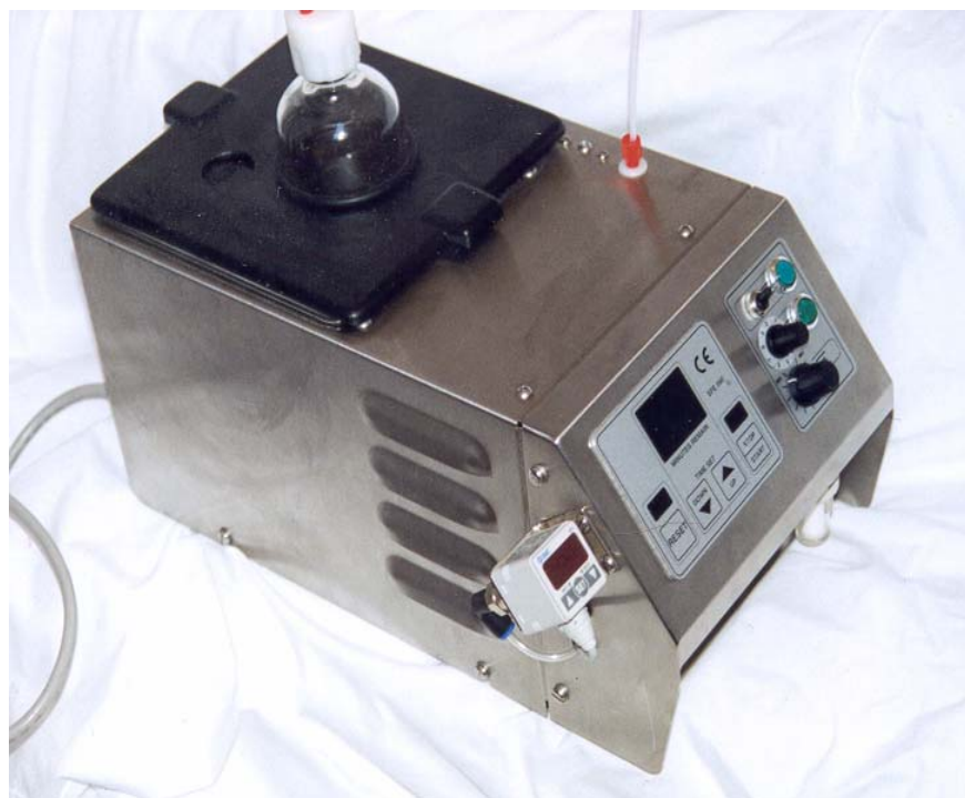
Figure 3. Ultrasonic Vacuum Degassing Unit
