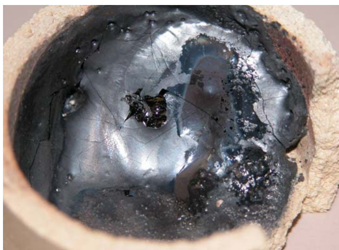
Figure 26 - MLS-1a simulant completely melted and partially vaporized after testing
