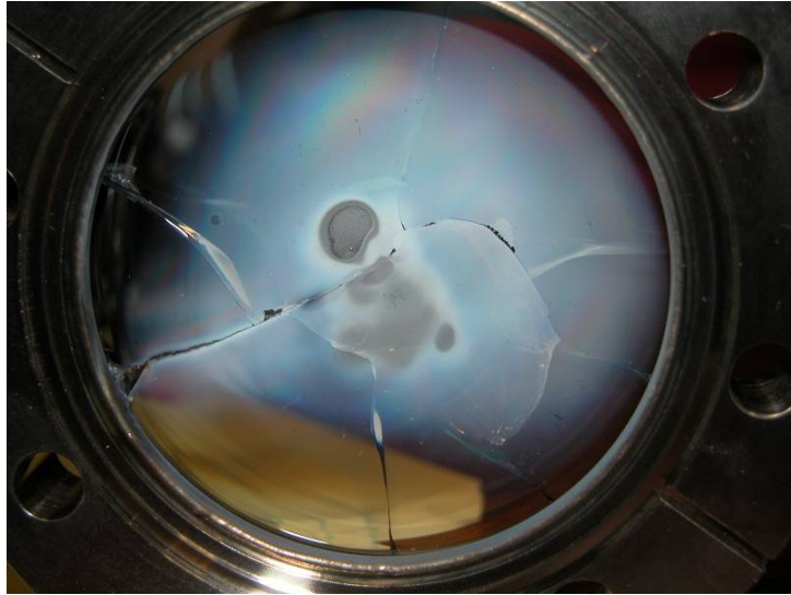
Figure 24 – Simulant condensation on glass vacuum seal flange
