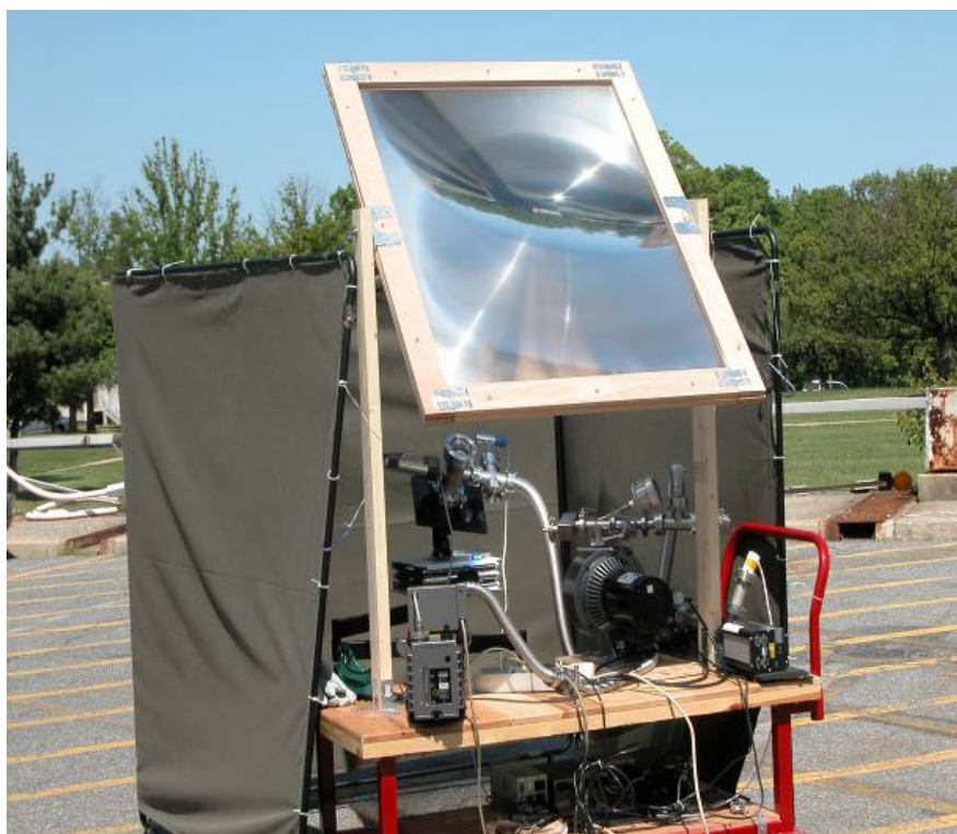
Figure 19 – Fresnel Lens Vacuum Pyrolysis Experimental Setup
