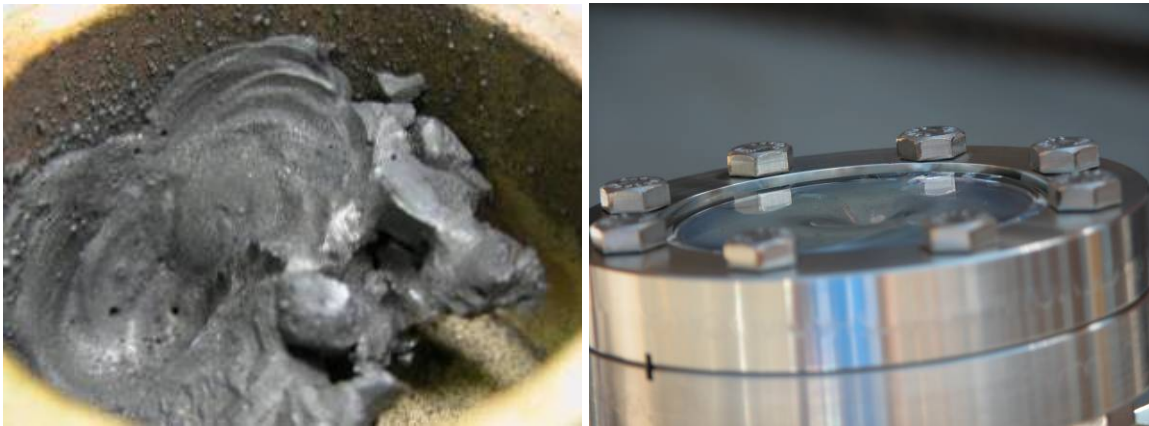
Figure 23 – (A) Melted Ilmenite with spatter and condensation on crucible walls. (B) Melted glass flange
