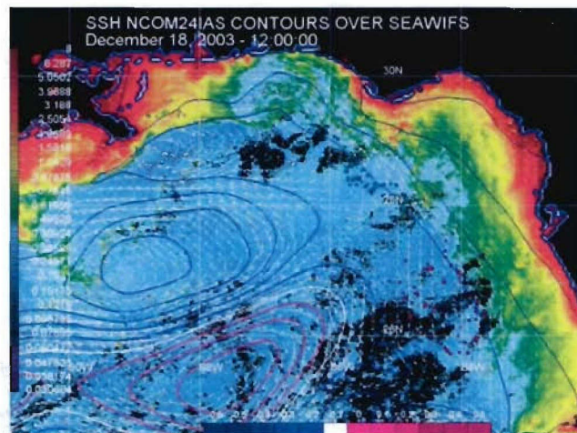
Figure 4- The SeaWIFS chlorophyll field and NCOM model are used to illustrate how coastal currents help define the chlorophyll distribution in coastal areas. The SSH are shown in the contours and the white and red dots represent particle that were seeded in the model.
