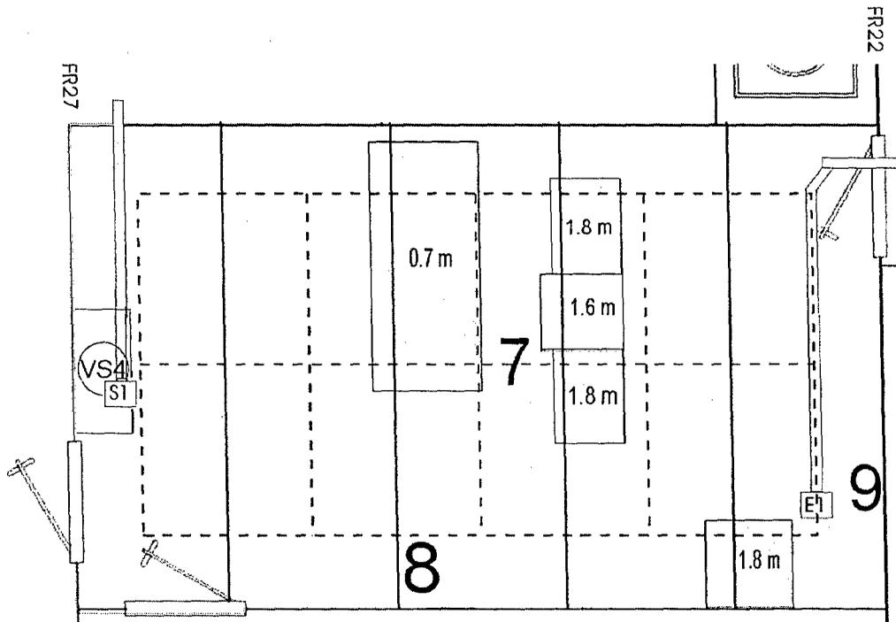
Fig. 4 — Layout of deck obstructions and source locations within 2<sup>nd</sup> deck magazine
