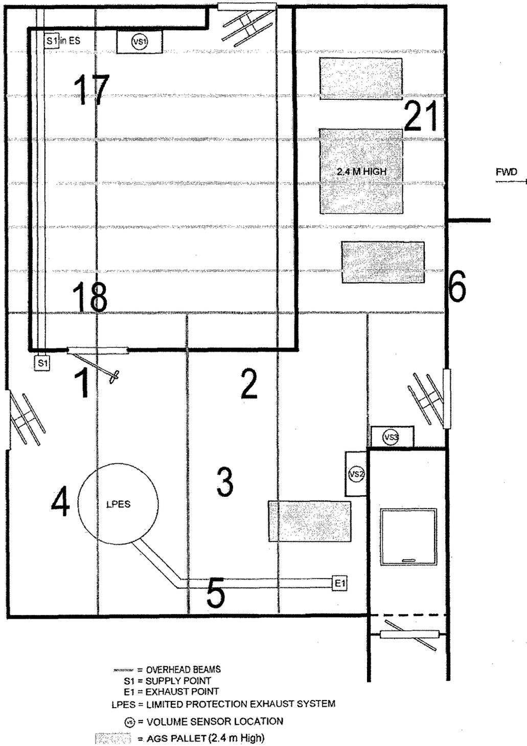
Fig. 3 — Layout of deck obstructions and source locations within 3<sup>rd</sup> deck magazine
