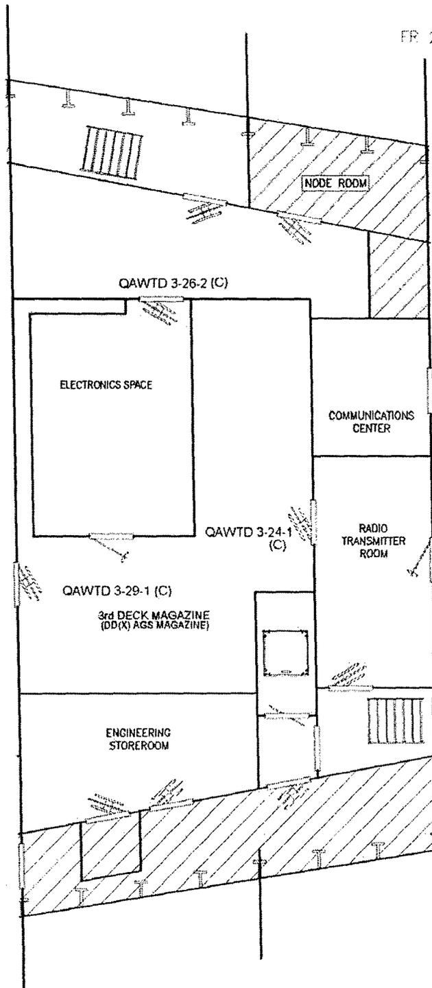
Fig. 1 — Layout of the spaces in the vicinity of the 3<sup>rd</sup> deck magazine
