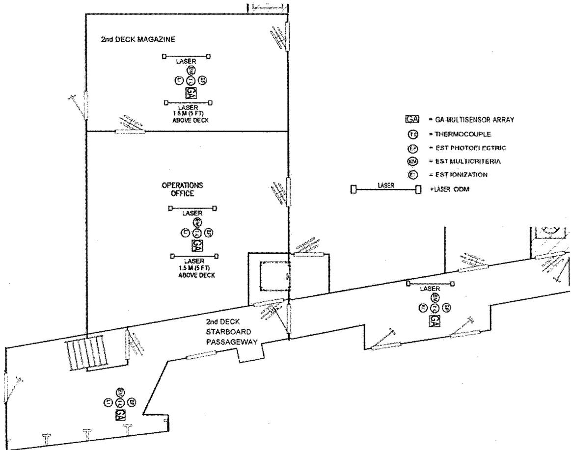
Fig. 12 — Locations of the GA sensor arrays, ODMs and spot-type detectors in 2<sup>nd</sup> deck test compartments
