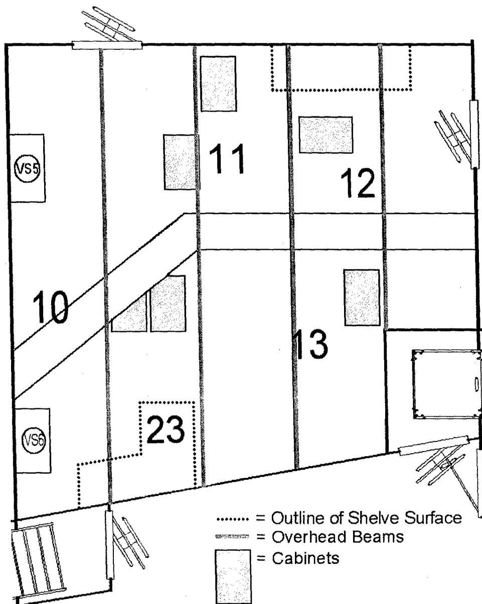
Fig. 5 — Layout of deck obstructions and source locations within 2<sup>nd</sup> deck operations office
