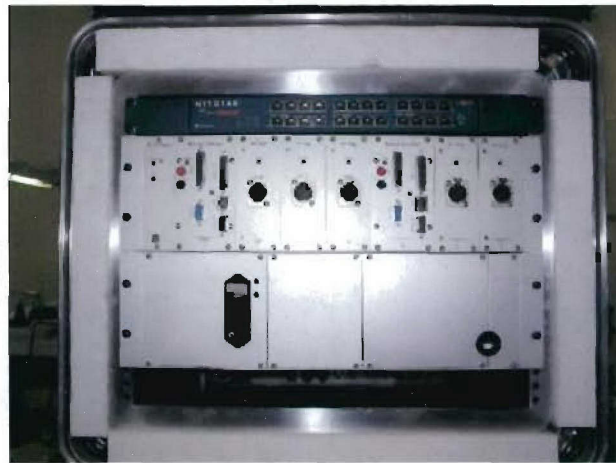
Figure 16. Nanomotor drive circuitry in the portable equipment rack.
