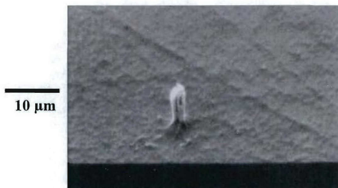
Figure 5.28. Scanning electron micrograph of a Br-IBAE etched GaSb wafer. This wafer was poorly polished and the etching has revealed polishing scratches and damage. Note that the micro-masked mesa shows the etching to be very anisotropic.
