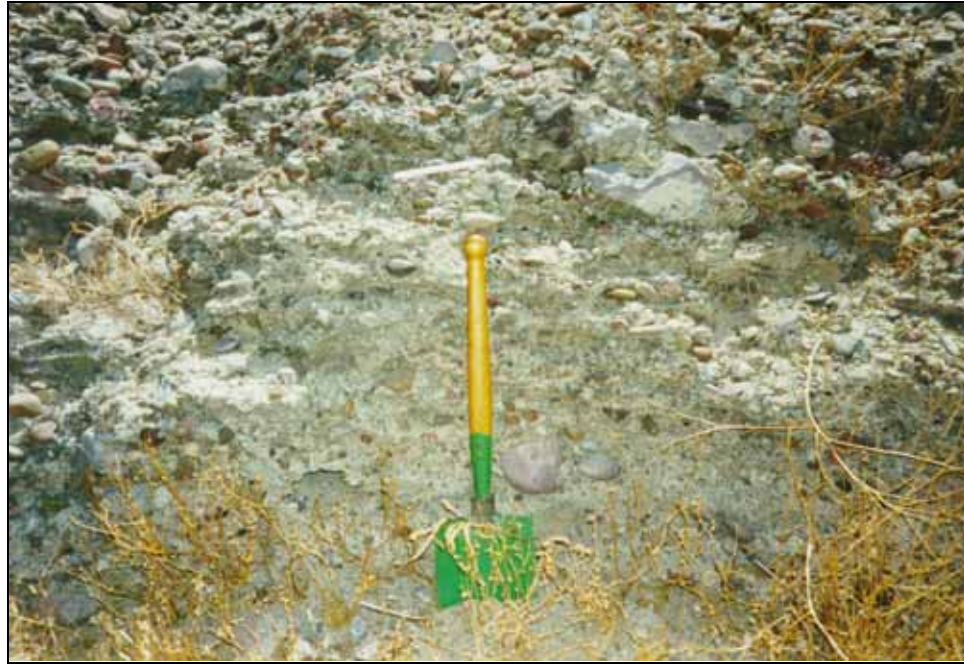
Figure 17. Calcium carbonate cemented Gila River fluvial gravels at Yuma Proving Ground.
