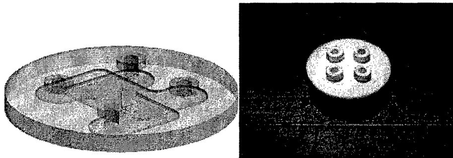
(a) Rendition of Internal Structure (b) Fabricated Heat Exchanger
