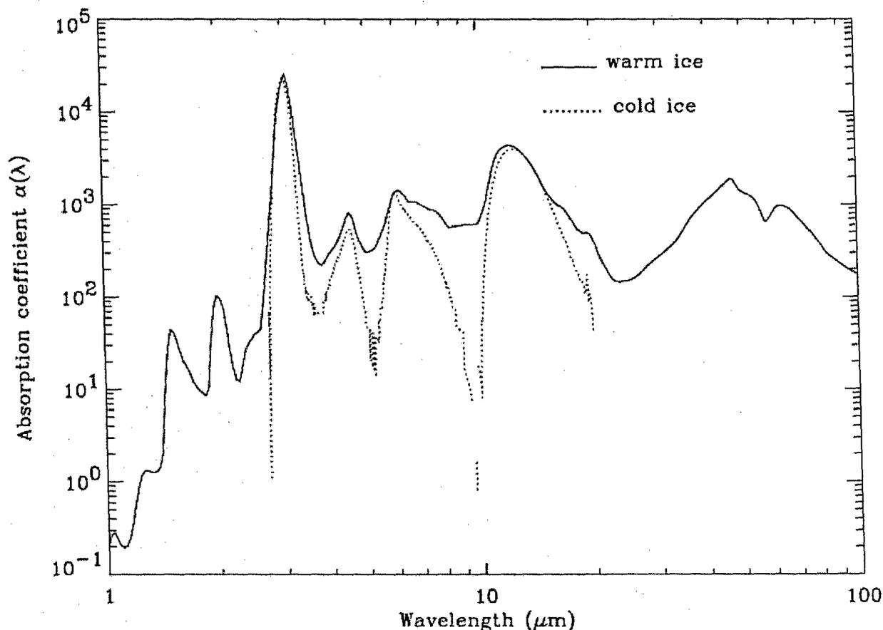
Figure 2. Absorption coefficient  $\alpha(\lambda)$  of warm (250K)<sup>6</sup> and cold (80K)<sup>8</sup> ice based on tabulations of Warren<sup>6</sup> and Hudgins et al.<sup>8</sup>
