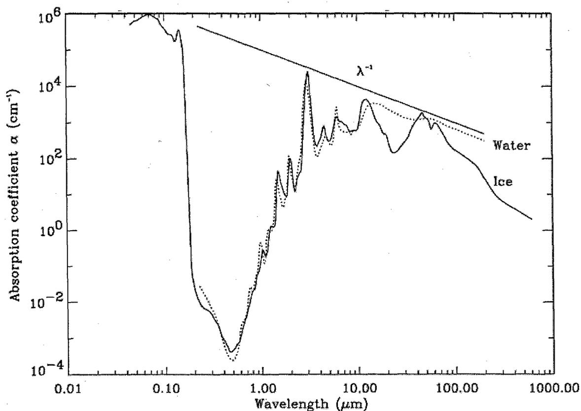
Figure 1. Absorption coefficient  $\alpha(\lambda)$  of water and ice from the ultraviolet to the far IR. Ice data are from Warren,<sup>6</sup> and water data are from Hale and Query.<sup>7</sup>
