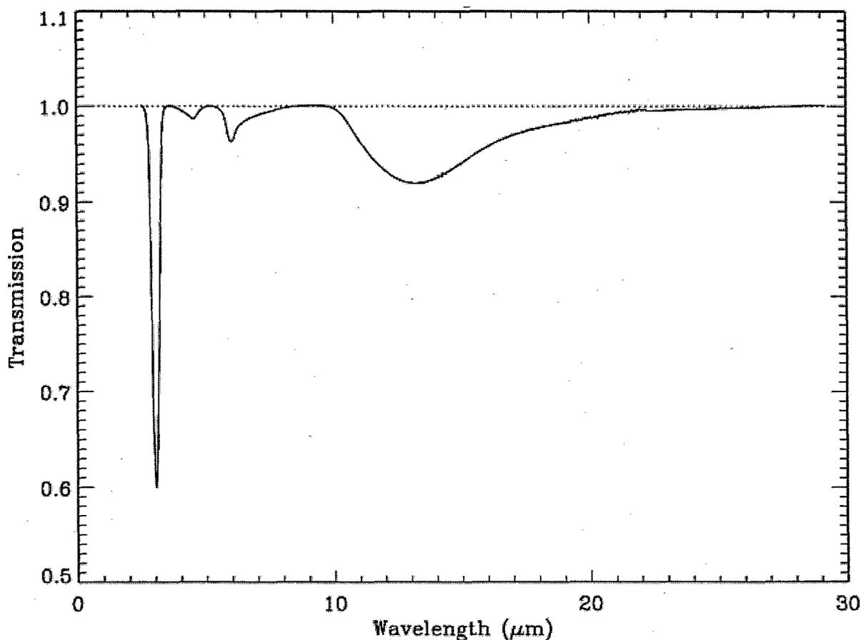
Figure 4. Transmission spectrum of a  $0.13\text{-}\mu\text{m}$ -thick film of ice deposited in vacuum onto a  $10\text{K}$  surface based on tabulations of the Jena group ([www.astro.uni-jena.de](http://www.astro.uni-jena.de)).
