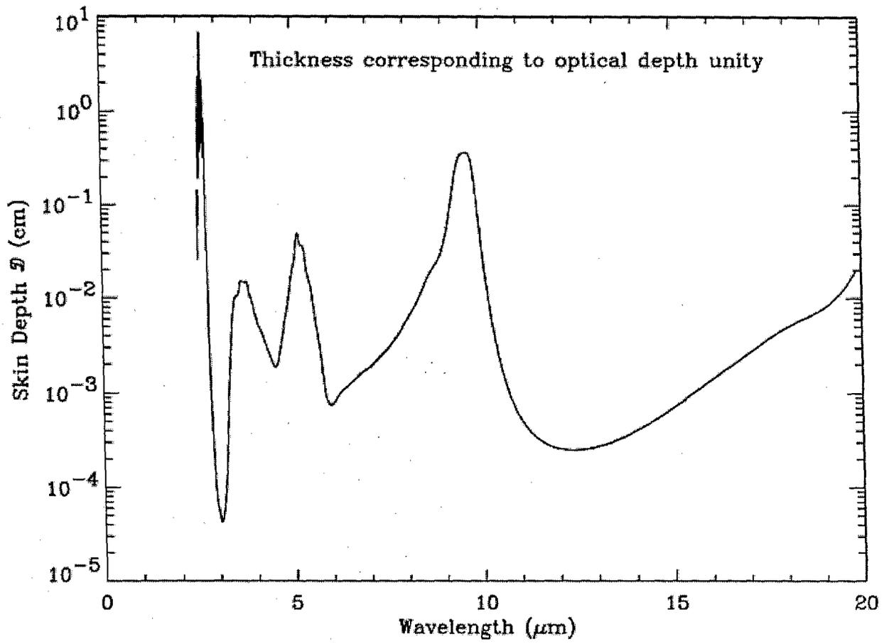
Figure 3. Skin Depth  $\mathcal{D}$  ( $1/\alpha$ ) of cryogenic(80K) ice based on tabulations of Hudgins et al.<sup>8</sup> The skin depth corresponds to an absorption optical depth of unity.
