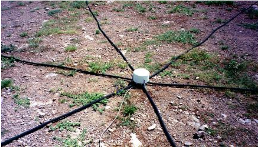
Figure 2. Chaparral Physics Model 2 microphone is used as the sensor for the array with six garden hoses used to filter and reduce wind noise.
