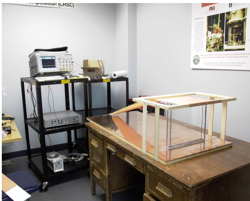
Figure 1: The antenna and some of the related equipment. An empty plexiglass container is placed in the parallel portion of the antenna to illustrate the placement of the agar target. Resistive end termination wires can be seen across the aperture.
