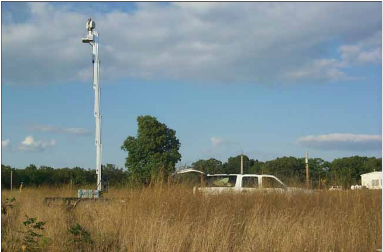
Figure C1. Trailer-mounted setup of Leica HDS3000 3D Laser Scanner elevated 7.62 m above Grass Site (viewed from southwest looking northeast, taken 26 July 2004)
