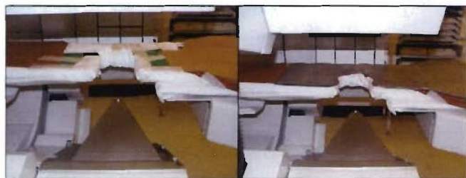
Fig. 2. A) Without Shielding B) With Shielding 5mm lead sheets were placed on the patient bed to simulate shielding. A ceiling mounted laser projected an x-y plane onto the dorsal side of the phantom, allowing for the accurate repositioning of the torso between scans.
