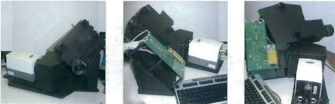
Figure 7: Several views, electronics exposed, of the NSTIS camera. The leftmost shows the system from the front; center view from the back; rightmost from the side.
