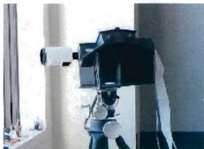
Figure 26: NSTIS camera fielded at NAVAIR China Lake facility. The system was fielded in a mobile configuration with tripod and telescopic imaging lens. Majority of data was collected through an open window on the upper floor of a large building.
