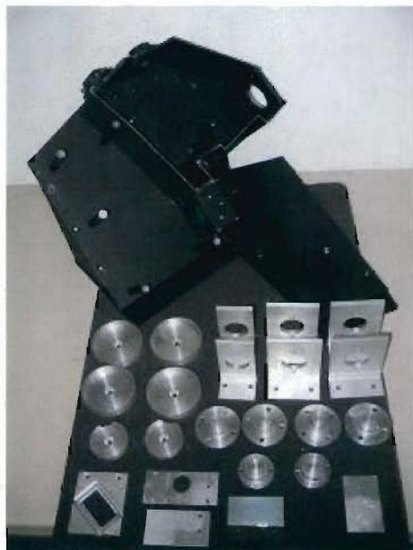
Figure 21: Main optical bench completed and displayed with uncoated optical mounting components.
