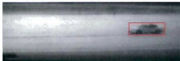
Figure 33: Image from localized datacube acquired by NSTIS with target box indicated in red that was used to train algorithm.
