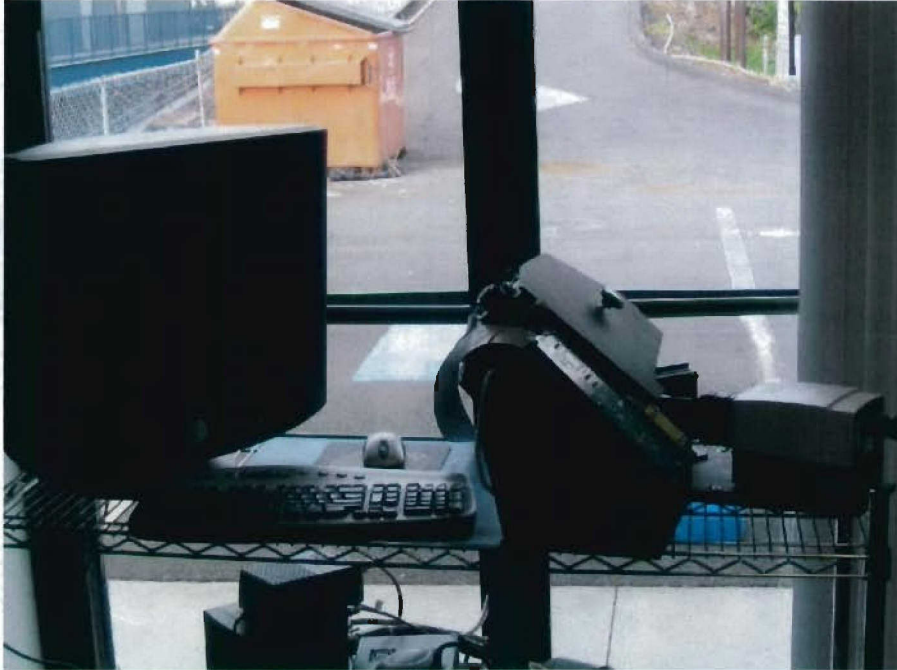
Figure 23: Completed NSTIS2 system deployed with PC in a mobile configuration. The system is shown imaging a natural scene through the window of building.
