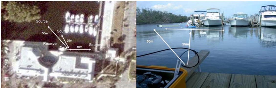
Figure 3. Sky and side view of the SeaTech marina, indicating the source and receiver locations (25 and 50 m ranges) during the experiments of January 2006.
