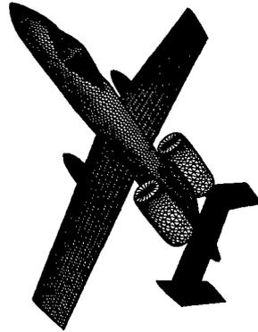
Figure 42: Surface triangulation of an aircraft-shaped object 50 wavelengths in size. The size of the smallest triangle is  $1.06 \times 10^{-6}$  wavelengths, and the size of the largest is  $2.86 \times 10^{-1}$  wavelengths.
