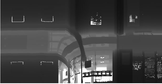
(a) The raw data of the laser scanner as depth image.
