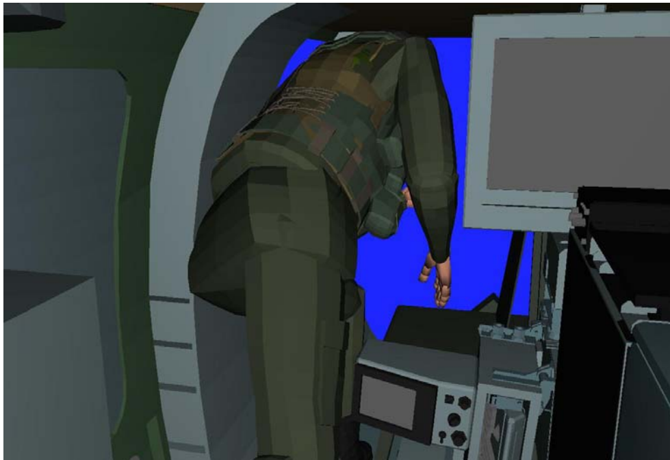
Figure 27. Large male figure leaving through space provided when workstation is folded down.
