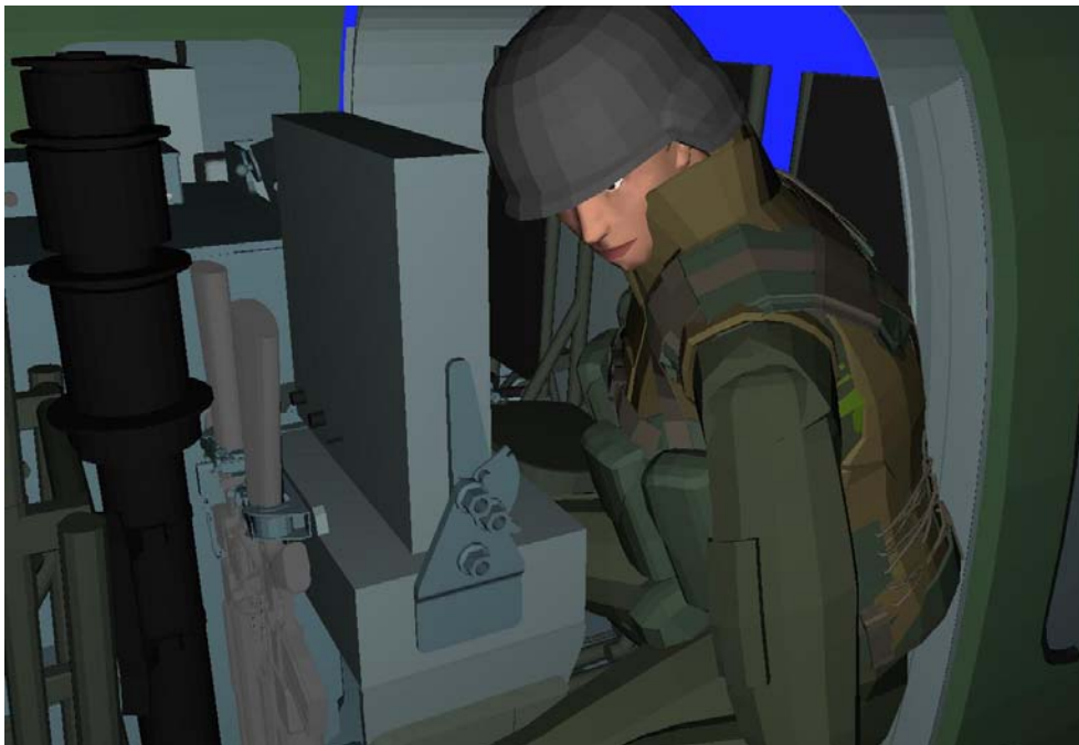
Figure 24. Restricted head space with monitor positioned upright.
