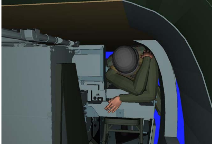
Figure 14. Large male figure positioning shoulders to leave over workstation.
