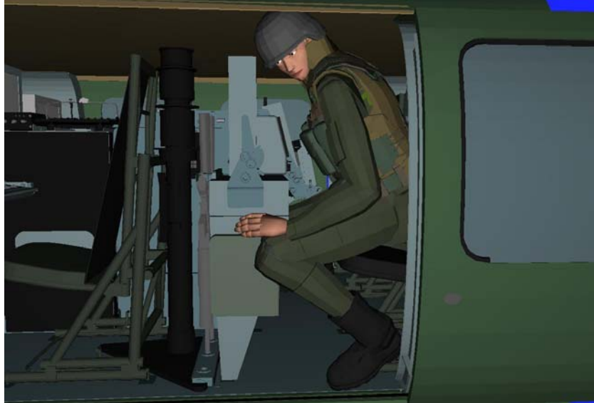
Figure 8. Human figure model sliding across rear seats.
