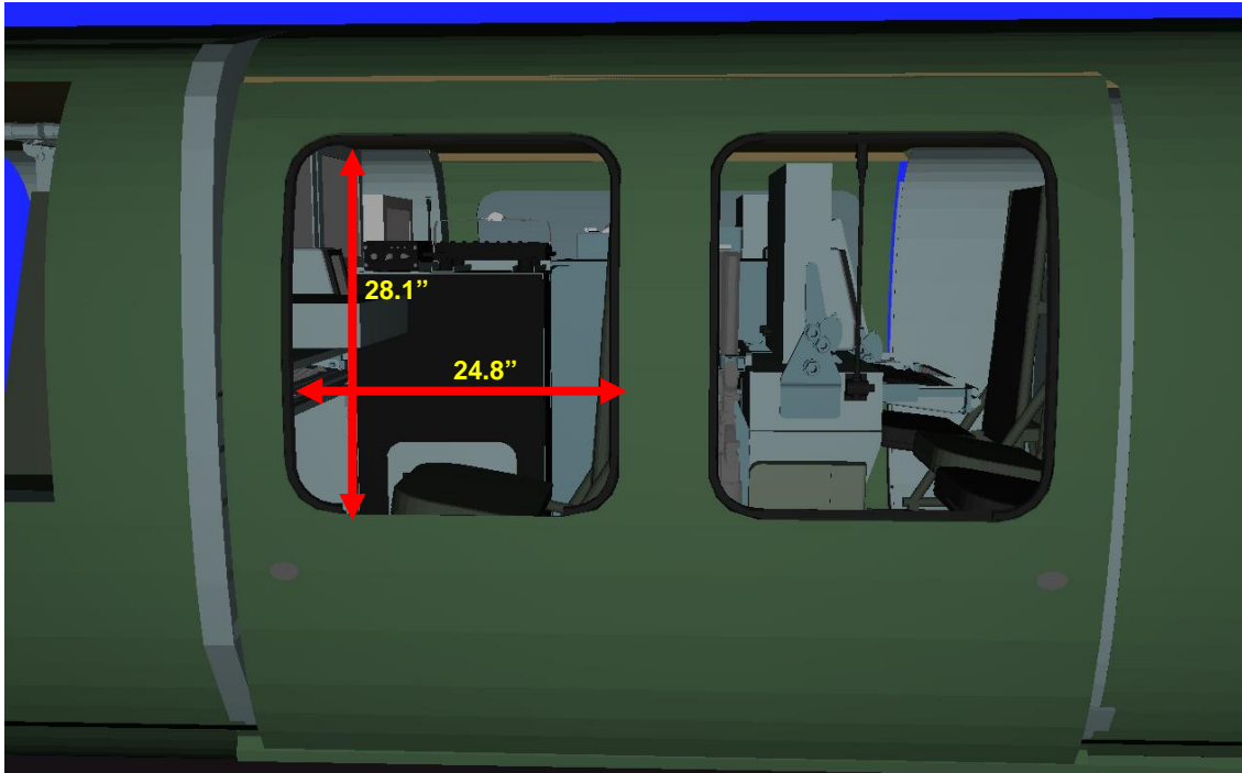
Figure 19. Dimensions of side cargo door window openings.
