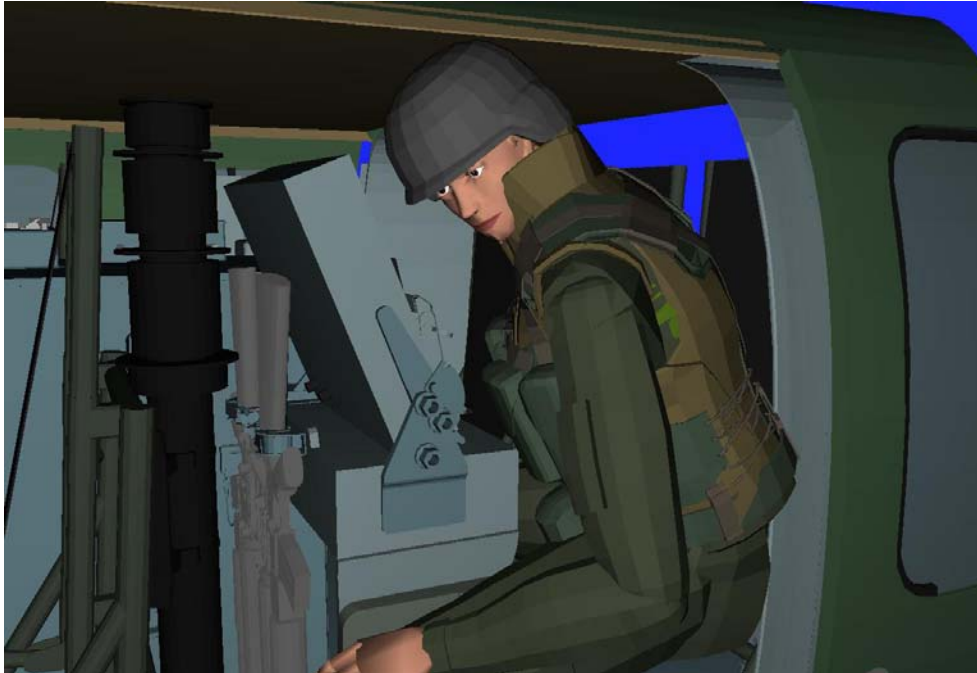
Figure 25. Additional head space provided by rotating monitor backward 20 degrees.
