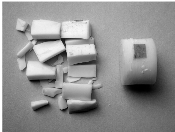
Fig. 18 Ceramic/composite sample after testing at 20.5 m/s.
