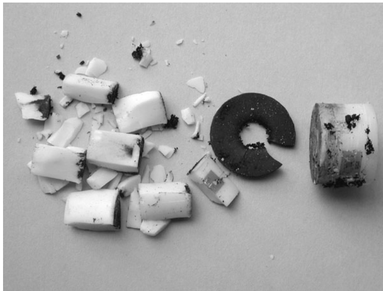
Fig. 23 Unconstrained ceramic/rubber/composite sample after testing at 20.5 m/s.
