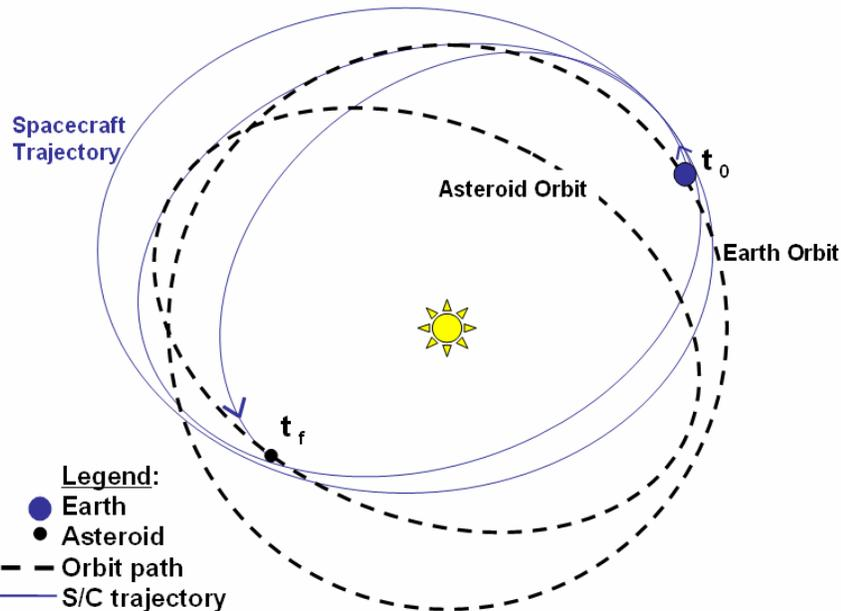
Figure 24 Earth to Asteroid Low Thrust Trajectory Representation
