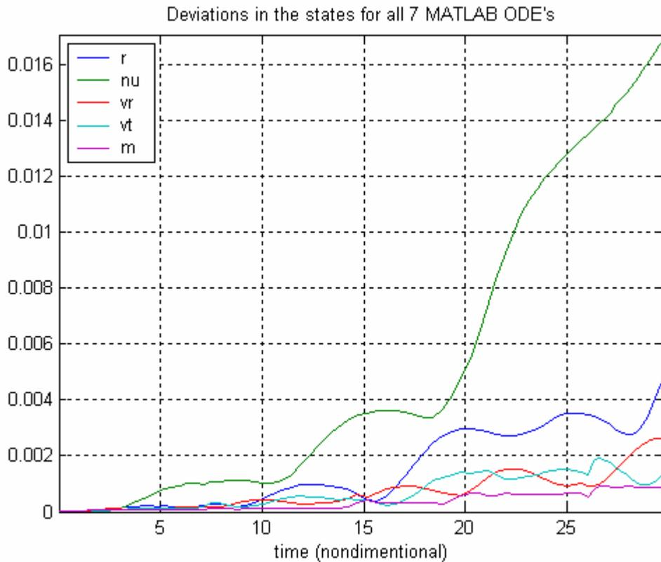
Figure 5 State deviations between ODE solvers over time
