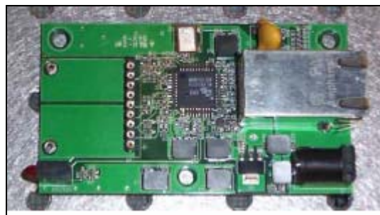
Figure 4. Modified ML6652RDK Media Converter (From Ref. [1]).
