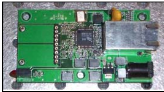
Figure 22. Modified ML6652RDK Media Converter (From Ref. [1]).
