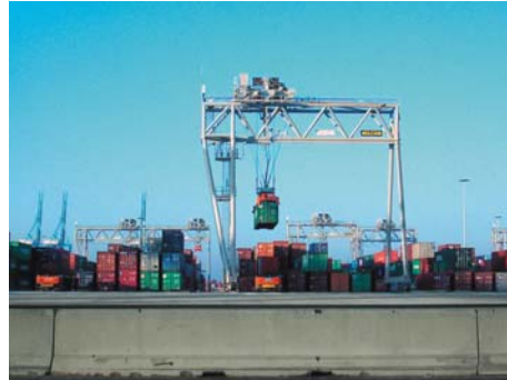
Figure 7. Automated Stacking Crane (ASC). (From: Kalmar Industries [2005]) ASC operating at ECT Delta terminal in Rotterdam
