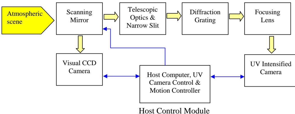
Figure 8 Schematic Block Diagram for LINUS (from Khoo)
