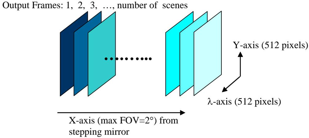
Figure 16 Hyper Spectral Data Cube Formed by LINUS Output (from Khoo)
